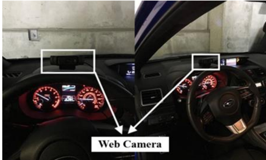
Fig. 12. Installing a camera near the dashboard to monitor driver status.
