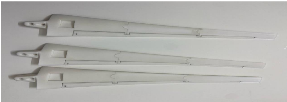
Fig. 4 Multi Cross-Section Three Blade With Flaps Printed in 4D Printer.
