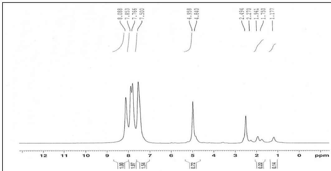
Fig (3) :  $^1\text{H-NMR}$  spectrum of compound [10].
