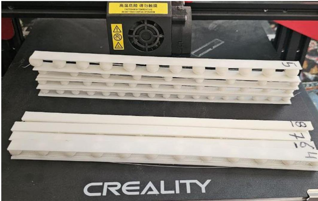
**Fig.4. Samples sandwich beam with spherical core used in experimental work.**
