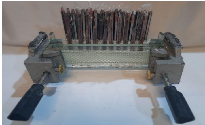
Fig.2. Installing and fixing the mold parts using the clamps
