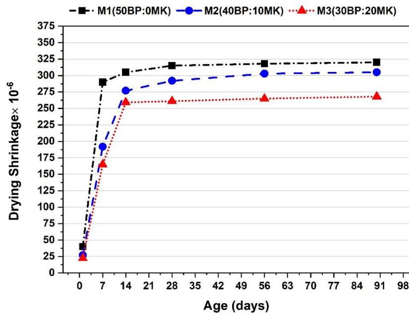
Fig. 12. Drying shrinkage of HVBP concrete mixtures
