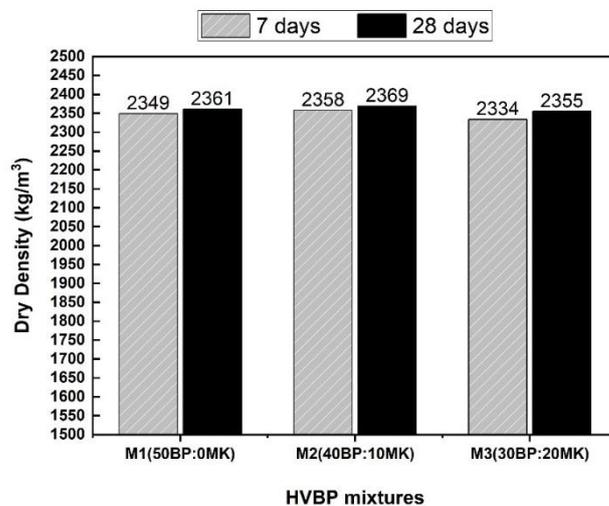
Fig. 7. Dry density of all HVBP concrete mixtures at 7 and 28 days
