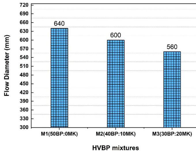
Fig. 5. Flow table results of the mixtures
