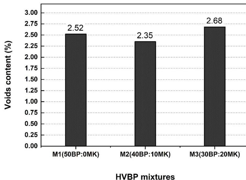
Fig. 8. Voids content of the mixtures at 28 days
