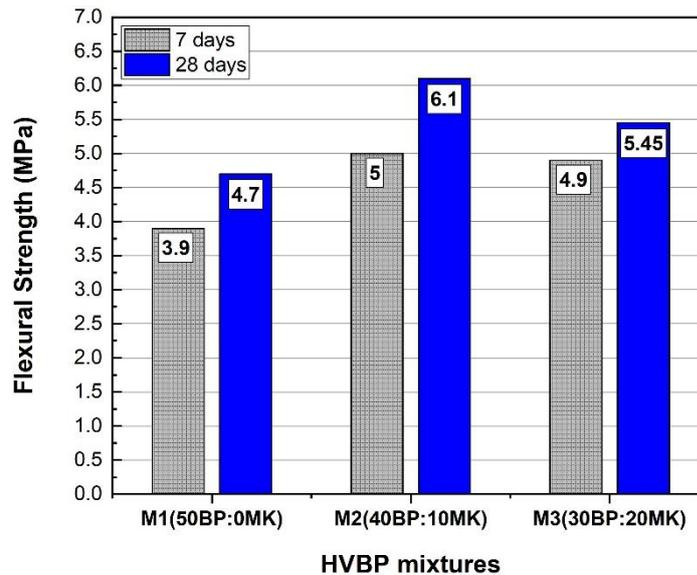
Fig. 10. Flexural strength of the mixtures at 7 and 28 days
