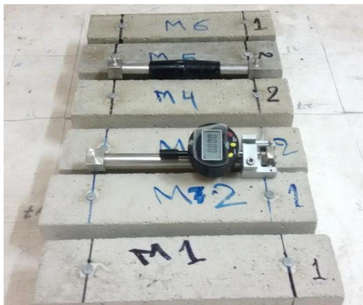
**Fig. 2. Specimens and approach of drying shrinkage test**
