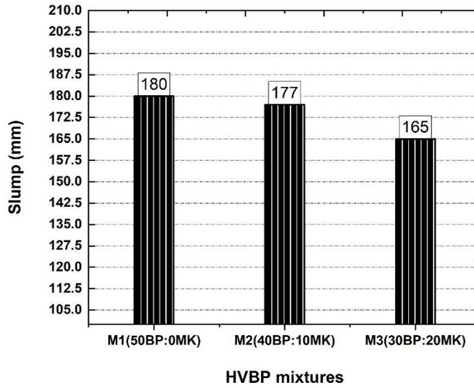
Fig. 4. Slump values of concrete mixtures
