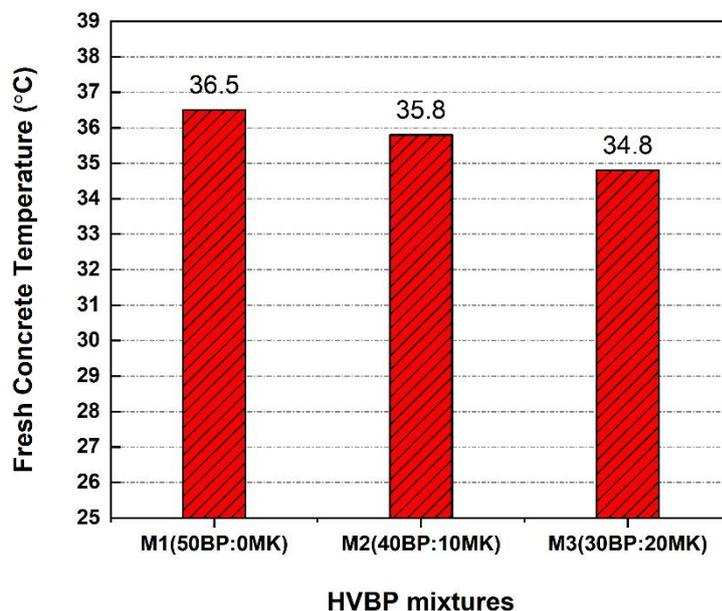
Fig. 3. Temperature of fresh concrete mixtures
