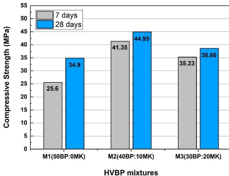
Fig. 9. Compressive strength of the mixtures at 7 and 28 days
