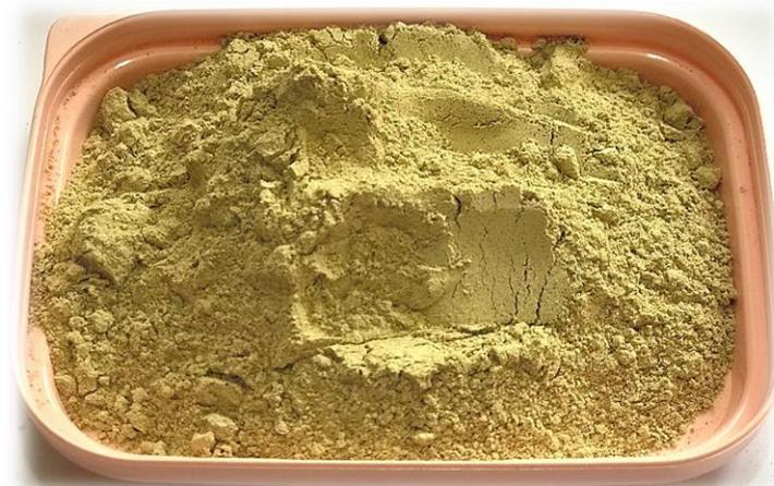
**Fig. 1. Waste clay brick powder**
