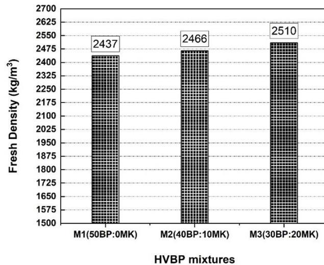
Fig. 6. Fresh density of the concrete mixtures
