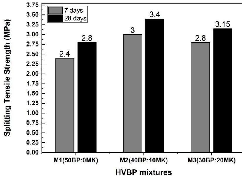
Fig. 11. Splitting tensile strength of the mixtures at 7 and 28 days
