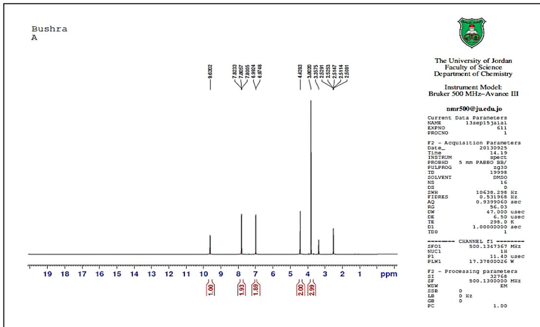
Figure.(4) <sup>1</sup>H NMR for compound(II<sub>2</sub>)
