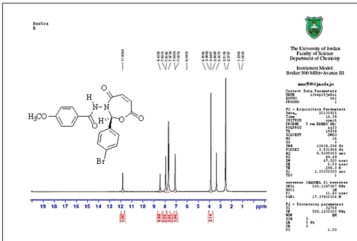
Figure.(7) <sup>1</sup>HNMR for compound(IV<sub>10</sub>)
