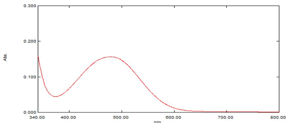
Fig (1) : Absorption spectra of ( $12.50\ \mu\text{g}\cdot\text{ml}^{-1}$ ) of Methyldopa with Thiamine Hydrochloride( $7.50 \times 10^{-7}$ )M , and  $\text{KIO}_4$ ( $5.00 \times 10^{-4}$ )M at room temperature and measured against blank solution.
