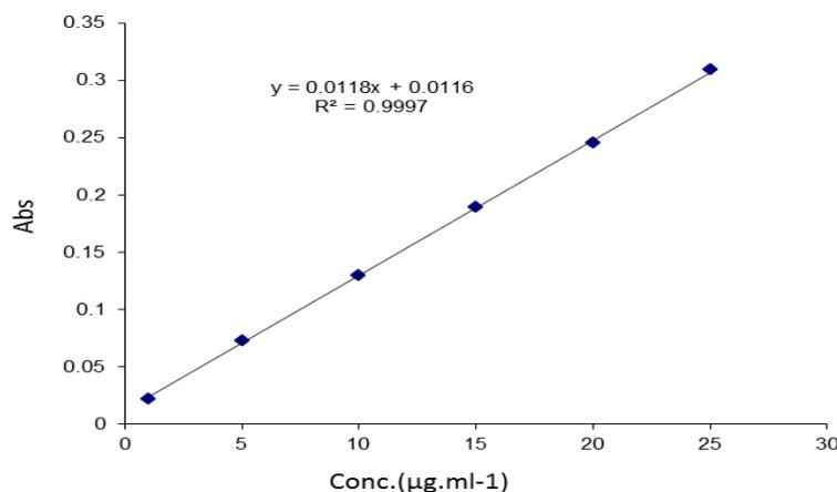
Fig (6) : Calibration graph for the determination of Methyl dopa
