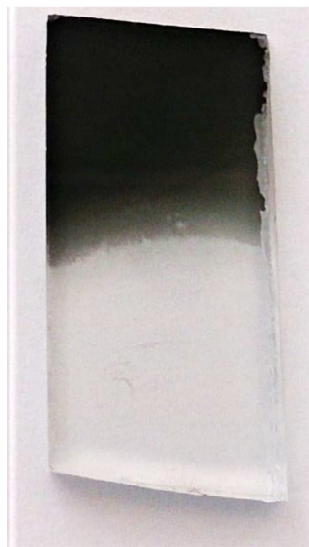
Figure 3. FTO surface coated with black film of poly-1.
