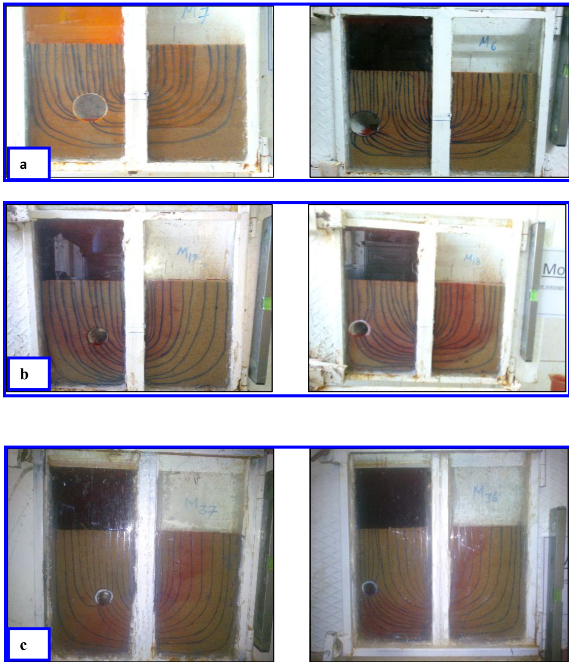
Fig.9 Effect Size of the Cavity on Shape of Flow line in Upstream Zone. (a) D=75\text{mm} , Yu./D=300 , (b) D=50\text{mm} , Yu./D=300 , (C) D=30\text{mm} , Yu./D=300 .
