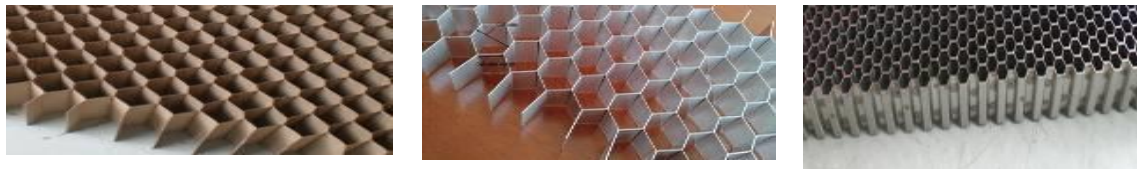
Fig. 1. Illustration of composite paper, aluminum and stainless steel honeycomb for construction application.
