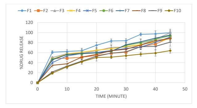
**Figure 2.** Percent of baclofen release of different ODT formulas in 900 ml phosphate buffer (pH 6.8) at 37°C, the results represent mean percent of drug released± SD (n=3).
