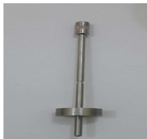
**Figure 3 : spindle 2. the spindle was used to measure the viscosity**
