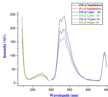
Figure (5) Ex-Em spectrum of Naphthalene after adding the sodium ions
