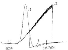
Fig.1. Spectra for the first derivative o an EPR signal of the anthracite sample measuring  $7x3x3 \text{ mm}^3$ ,  $\mathbf{X} \perp \mathbf{H_1}$  without (1) and with AFC when  $\mathbf{H_0}$  is increasing (2) or decreasing (3);  $P_1 = 3$  mW, the marks are given every 0.1 mT
