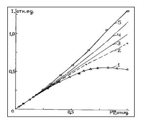
Fig.2. Intensity I of the EPR line as a function of the microwave radiation power  $P_1^{1/2}$  for the anthracite sample with the volume 0.5 mm<sup>3</sup> (1), for ruby (2), linear dependence of I on  $P_1^{1/2}$  (3) for the spectral carbon powder (4), for the anthracite powder in toluene(5)
