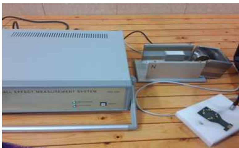
Fig. (5): Set-up and photograph illustrate the Hall effect.
