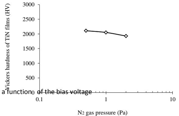
Fig.6. Vickers hardness of TiN films as a function of N<sub>2</sub> gas pressure.
