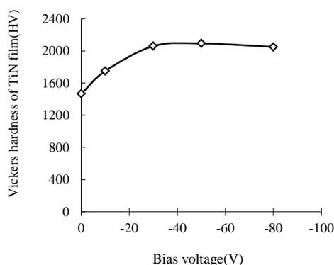
Fig.3. Vickers hardness of TiN films as a function of the bias voltage.
