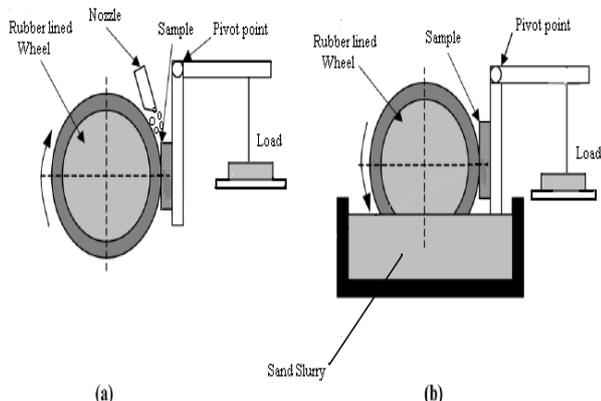
Fig.2. Schematic illustration of the (a) dry and (b) wet rubber wheel abrasive wear tests.
