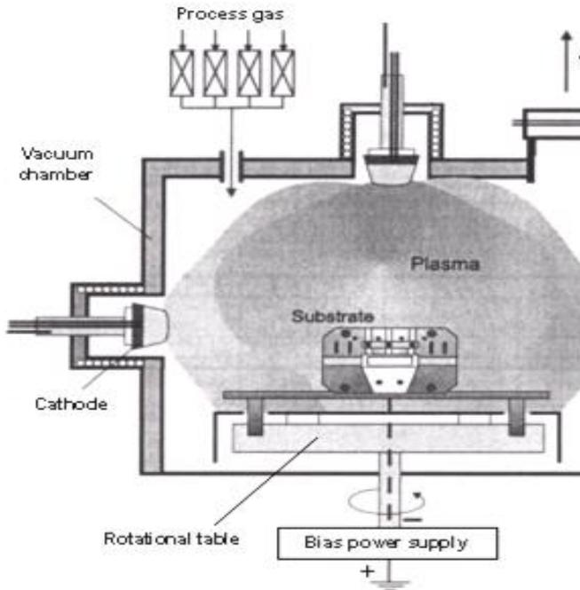
Fig.1. Schematic illustration of the apparatus for arc ion plating.
