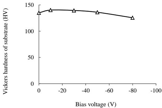
Fig.4. Vickers hardness of the substrate as a function of the bias voltage
