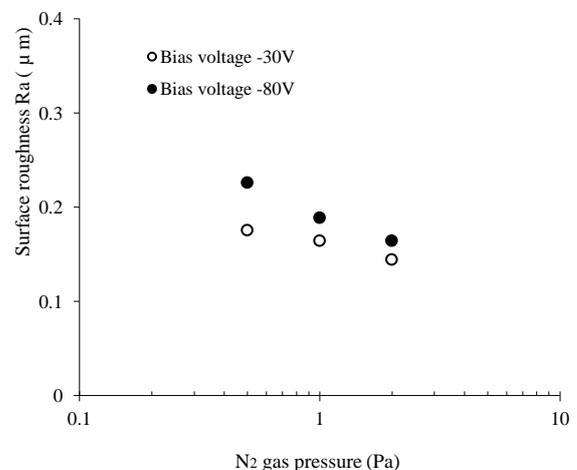
Fig.7. Effect of N<sub>2</sub> gas pressure on the surface roughness of TiN films.
