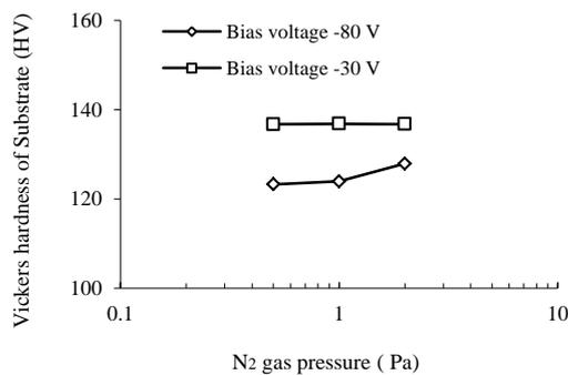
Fig.5. Vickers hardness of the substrate as a function of N<sub>2</sub> gas pressure.
