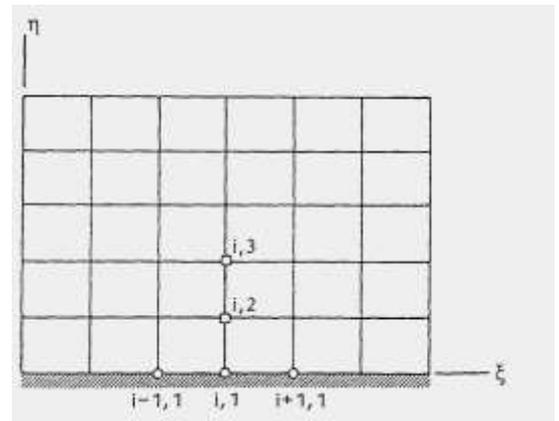
**Figure (3) Grid points for upper cowl surface in computational domain.**
