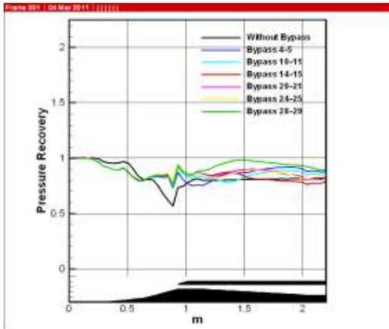
**Figure (10) Pressure recovery variation along Intake axis for all cases.**
