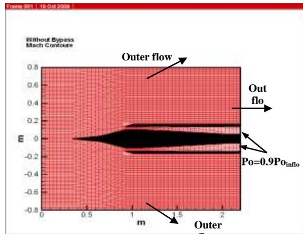
Figure (5) the outer flow boundary shown on the air intake.
