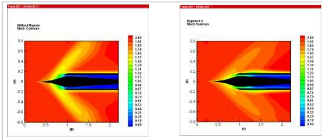
**Figure (8) Mach contours for the full geometry inlet with and without bypass Technique**
