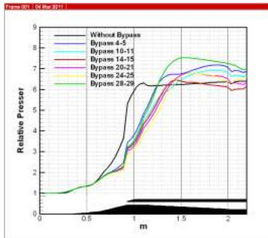
**Figure (12) Relative Pressure Variation along intake for all cases.**
