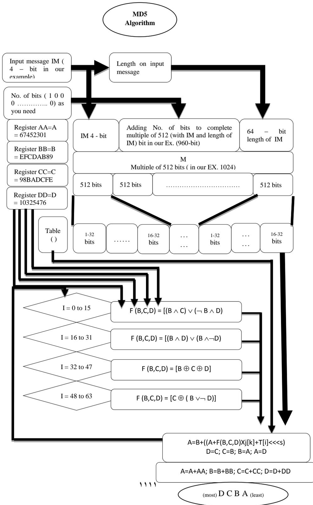
Figure (1) MD5 algorithm flowchart
