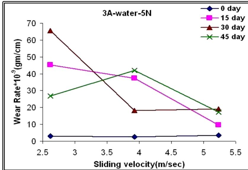
Figure (9) Wear Rate vs. Sliding Velocity for Blend (A) after Immersion in H<sub>2</sub>O.
