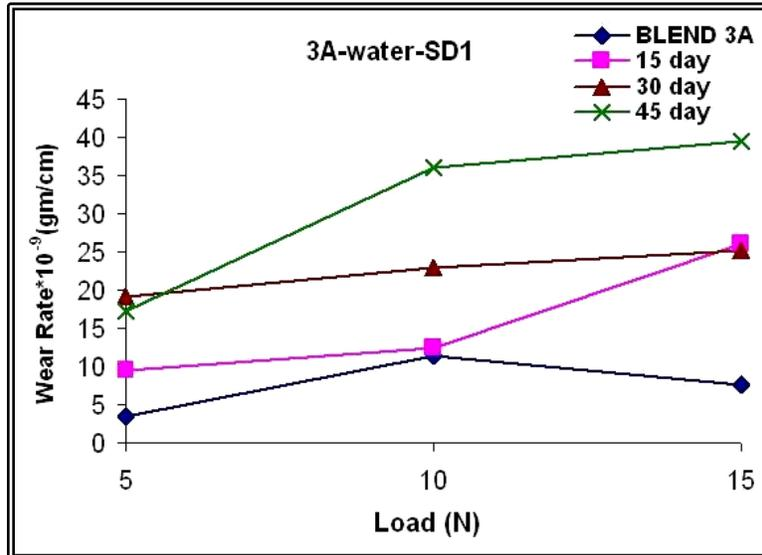
Figure(3) Wear Rate vs. Load for Blend (A) after Immersion in H<sub>2</sub>O.
