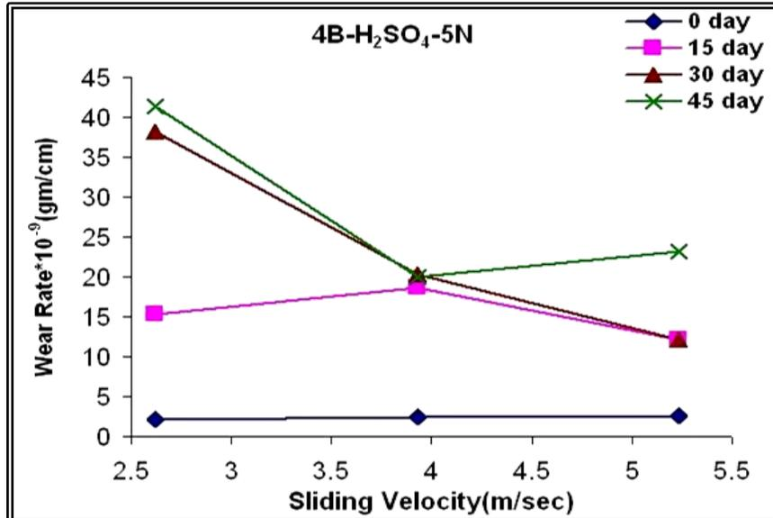
Figure (10) Wear Rate vs. Sliding Velocity for Blend (B) After Immersion in H<sub>2</sub>SO<sub>4</sub>.
