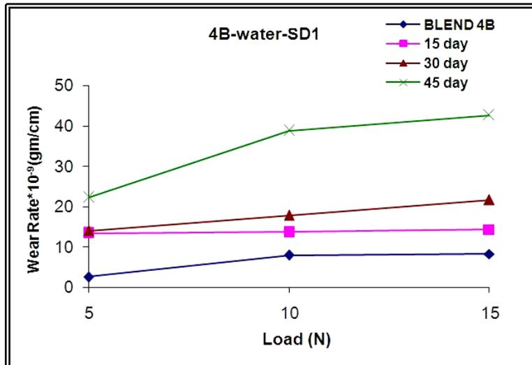
Figure (6) Wear Rate vs. Load for Blend (B) after Immersion in H<sub>2</sub>O.
