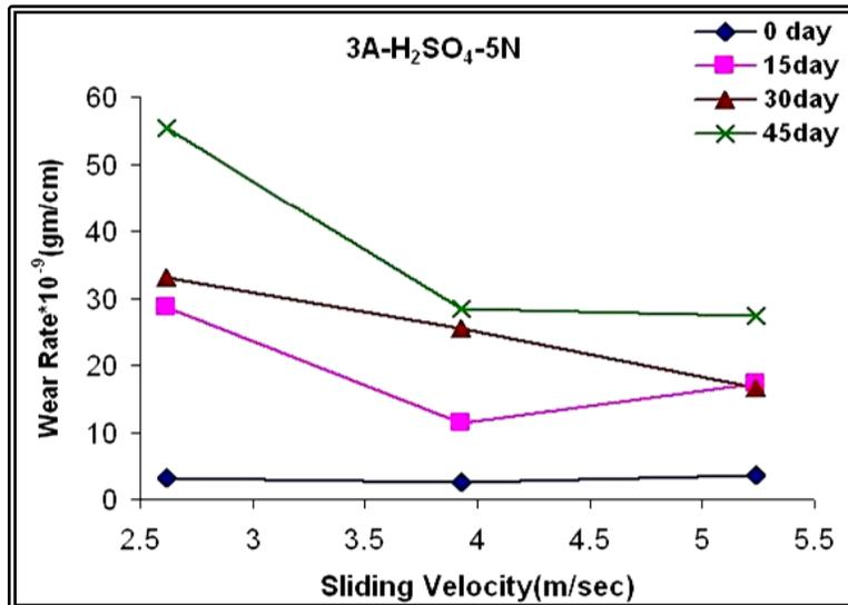
Figure (7) Wear Rate vs. Sliding Velocity for Blend (A) after Immersion in H<sub>2</sub>SO<sub>4</sub>.
