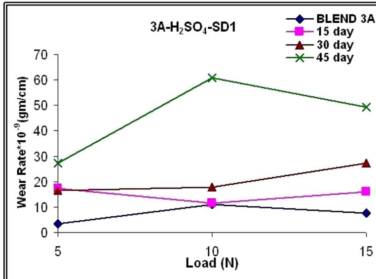
Figure (1) Wear Rate vs. Load for Blend (A) after Immersion in H<sub>2</sub>SO<sub>4</sub>.
