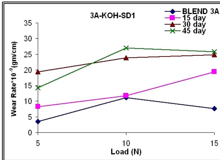
Figure (2) Wear Rate vs. Load for Blend (A) after Immersion in KOH.
