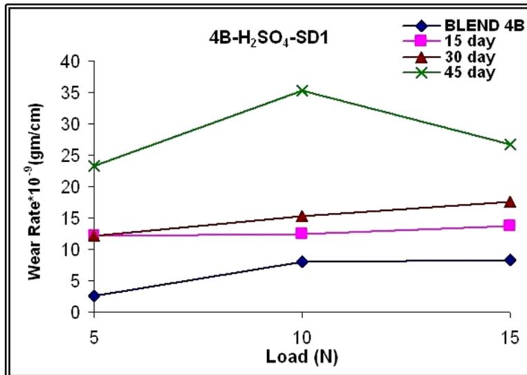
Figure (4) Wear Rate vs. Load for Blend (B) after Immersion in H<sub>2</sub>SO<sub>4</sub>.
