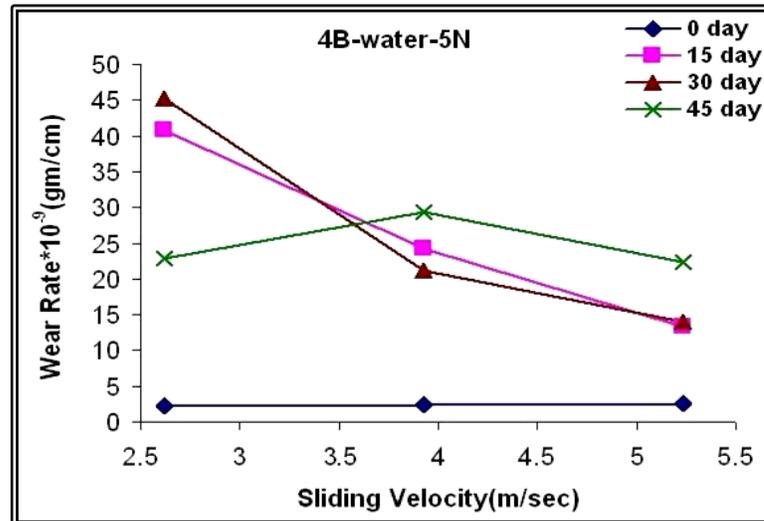
Figure (12) Wear Rate vs. Sliding Velocity for Blend (B) After Immersion in H<sub>2</sub>O.
