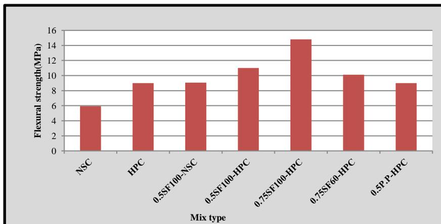
Figure (6) Flexural strength for all types of concrete at 60 days. age
