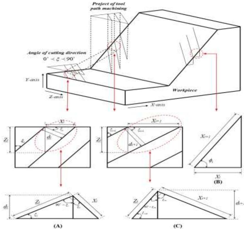
Figure (12 A,B and C) shows how step over is calculated in each plane if the angle of cutting direction  $0^\circ < \xi < 90^\circ$ : (A) explains step over in horizontal plane for  $(0^\circ < \xi < 90^\circ)$ . (B) explains the geometrical shape to find  $X_{i+1}$ .(C) explains step over in inclined plane for  $(0^\circ < \xi < 90^\circ)$ .
