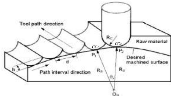
Figure (3 b) Scallop heights for a convex machined surface
