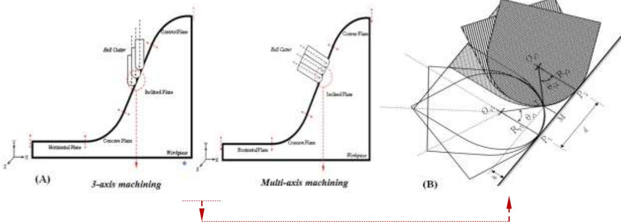
Figure.(7 A and B). Describes scallop height in inclined plane by using ball cutter for three and multi-axis machining.
