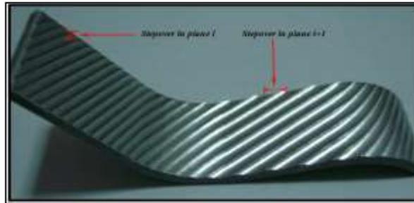
Figure (11) The magnitude of step over is change along the inclined plane when the angle of cutting direction  $0^\circ < \xi < 90^\circ$ .
