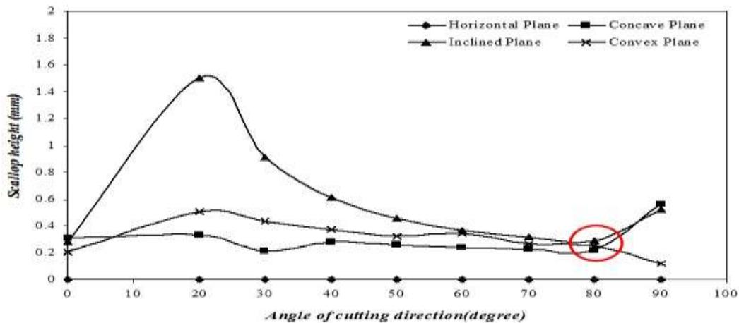
Figure.(19). Best cutting direction angle for each plane by using torus cutter.
