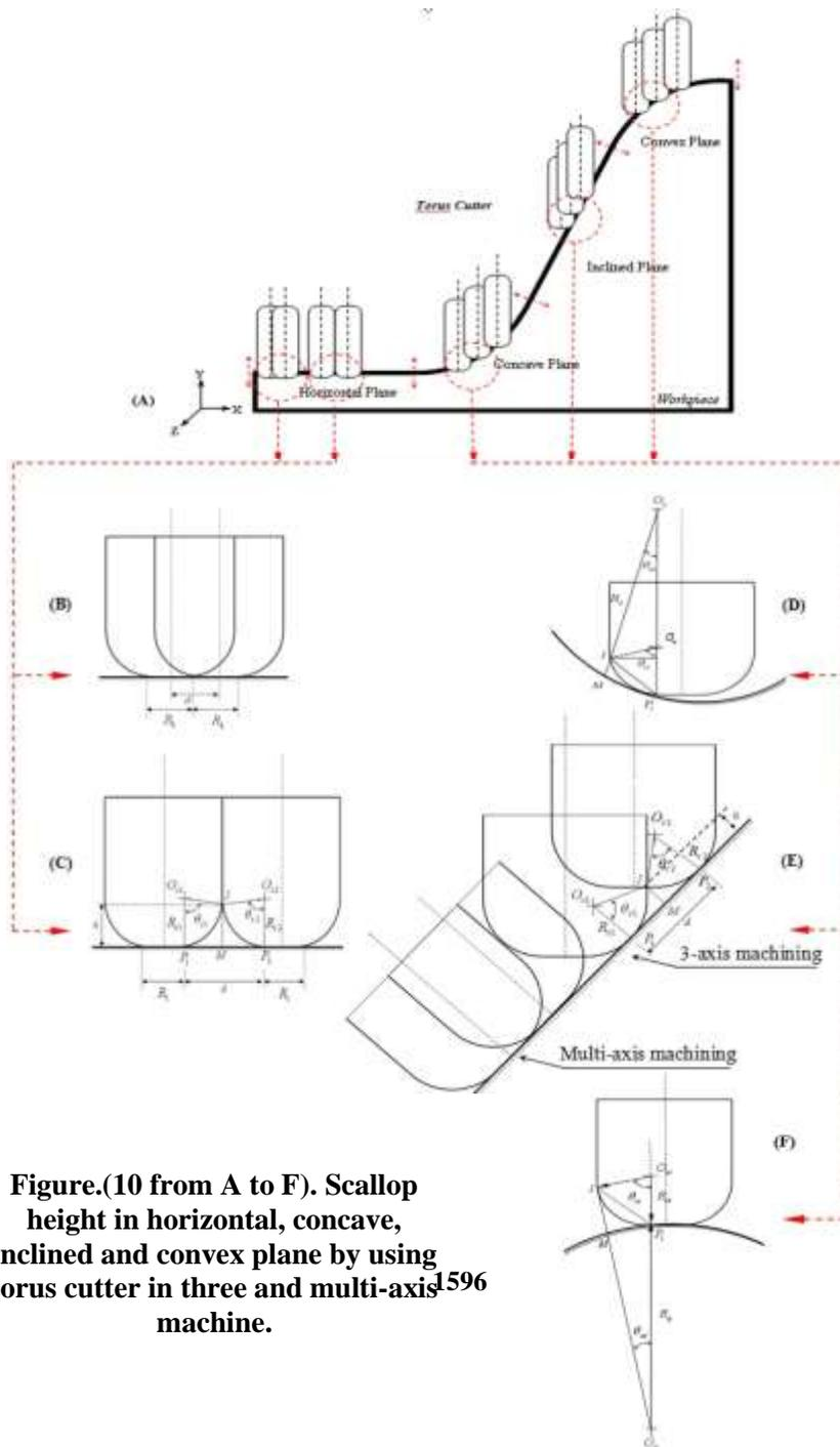
Figure.(10 from A to F). Scallop height in horizontal, concave, inclined and convex plane by using torus cutter in three and multi-axis machine.
