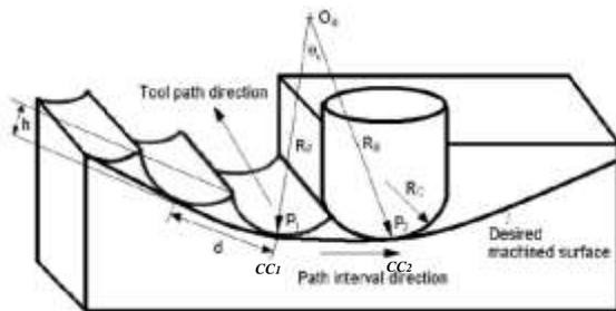
Figure (3a) Scallop heights for a concave machined surface.
