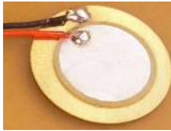
Figure (4) The piezoelectric sensor (Diameter = 15mm).
