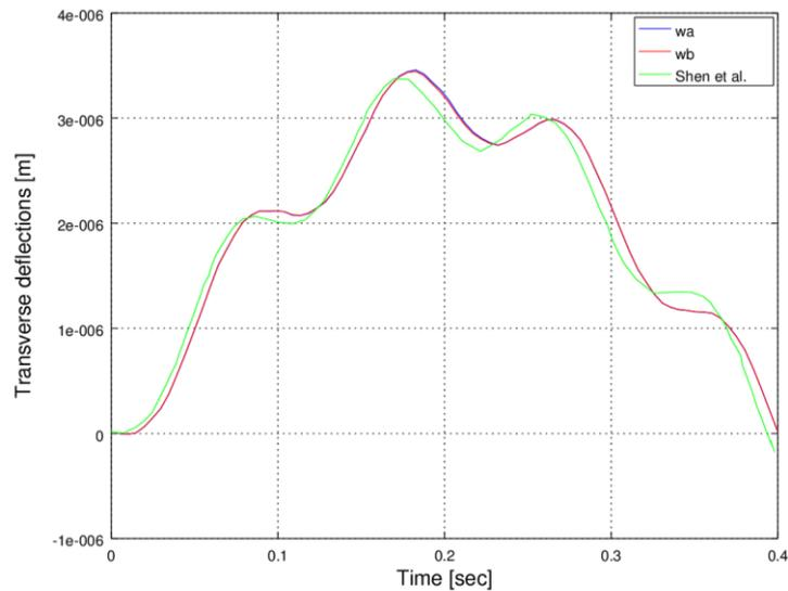
**Fig. 3 e Comparison of mid-span deflection  $w(t)$  of Shen *et al.*'s (2011) example to  $w_a(t)$  and  $w_b(t)$  given by the present model corresponding to a 1 Newton force crossing the beam at 10 m/sec**
