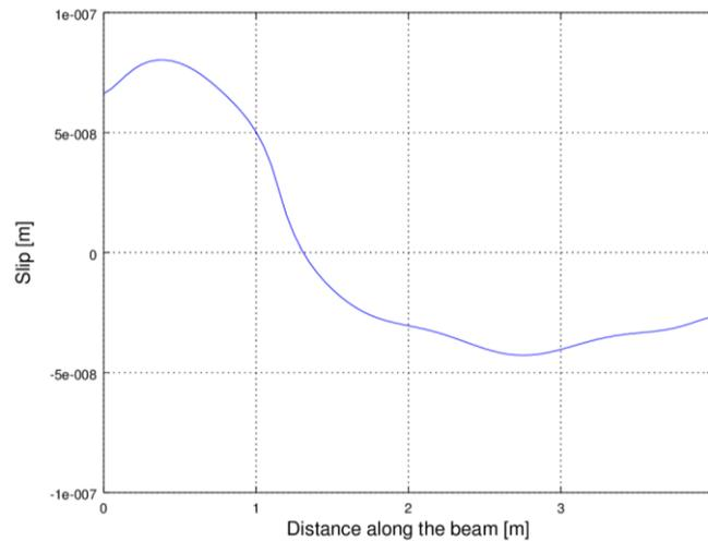
**Fig. 3 g** The slip field of Shen *et al.*'s (2011) example corresponding to a 1 Newton force crossing the beam at 10 m/sec at time 0.12 sec, as given by the present model
