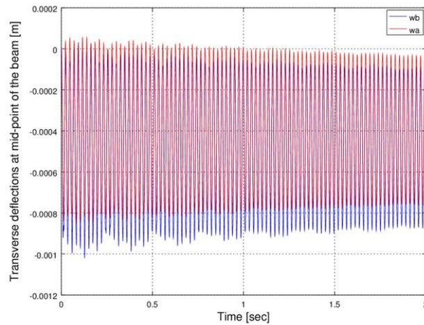
**Fig. 7 a** Dynamic mid-span transverse deflections of the numerical beam of 5 m length, the lower layer of which was fixed at both ends due to a uniform step 1 kN load, for a period of 2 seconds
