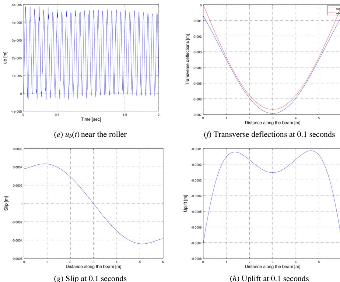
**Fig. 6 c-h Dynamic responses of the numerical simply supported beam of 6 m length with  $K_n = 0.5 \times 10^8$  N/m and  $K_s = 10^8$  N/m due to a uniform step 1 kN load**
