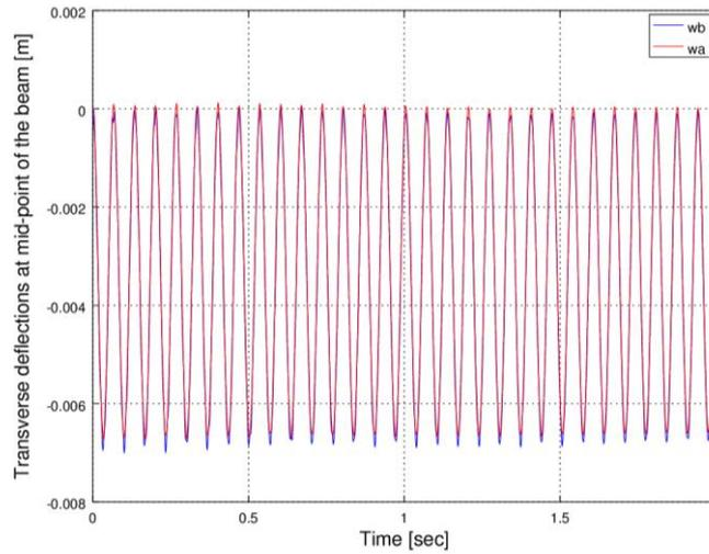
**Fig. 6 a** Dynamic mid-span transverse deflections of the numerical simply supported beam of 6 m length with  $K_n = 0.5 \times 10^8$  N/m and  $K_s = 10^8$  N/m due to a uniform step 1 kN load, for a period of 2 seconds
