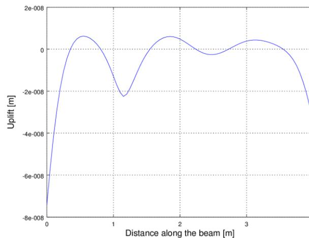
**Fig. 3 h** The uplift field of Shen *et al.*'s (2011) example corresponding to a 1 Newton force crossing the beam at 10 m/sec at time 0.12 sec, as given by the present model
