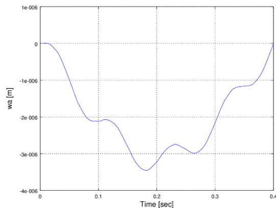
**Fig. 3 c** The mid-span  $w_a(t)$  of Shen *et al.*'s (2011) example corresponding to a 1 Newton force crossing the beam at 10 m/sec as computed by the present model
