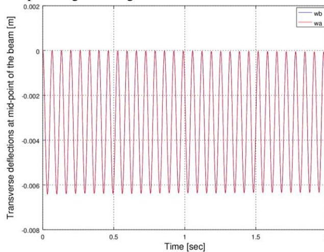
**Fig. 5 a Dynamic mid-span transverse deflections of the numerical simply supported beam of 6 m length with  $K_n = 10^{10}$  N/m and  $K_s = 10^8$  N/m due to a uniform step 1 kN load, for a period of 2 seconds**
