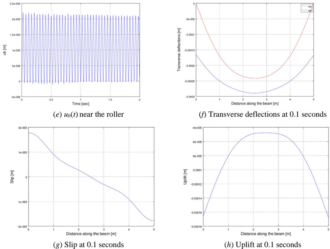
**Fig. 4 c-h Dynamic responses of the numerical simply supported beam of 5 m length due to a uniform step 1 kN load**
