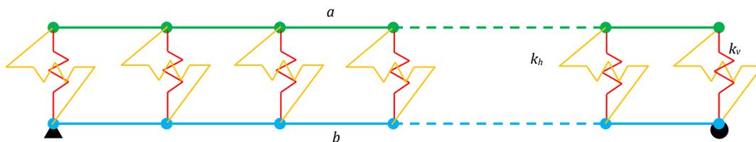
Fig. 1 A one-dimensional finite element model of a partial interaction composite beam
