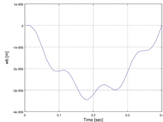
**Fig. 3 d** The mid-span  $w_b(t)$  of Shen *et al.*'s (2011) example corresponding to a 1 Newton force crossing the beam at 10 m/sec as computed by the present model
