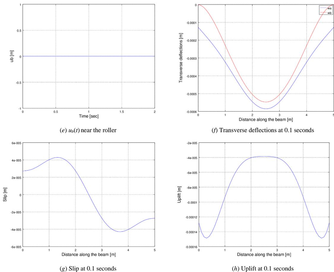
**Fig. 7 c-h Dynamic responses of the numerical beam of 5 m length, the lower layer of which was fixed at both ends due to a uniform step 1 kN load**
