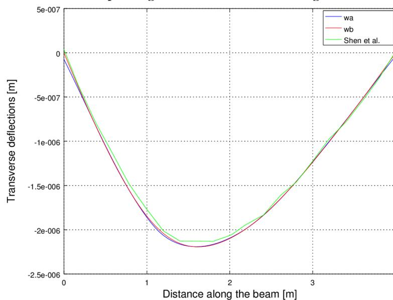
**Fig. 3 f Comparison of transverse deflection  $w(x)$  of Shen *et al.*'s (2011) example to  $w_a(x)$  and  $w_b(x)$  given by the present model corresponding to a 1 Newton force crossing the beam at 10 m/sec, exactly at 0.12 seconds**
