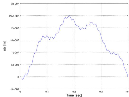
**Fig. 3 b** The variation of  $u_b(t)$  near the roller support of Shen *et al.*'s (2011) example corresponding to a 1 Newton force crossing the beam at 10 m/sec as computed by the present model
