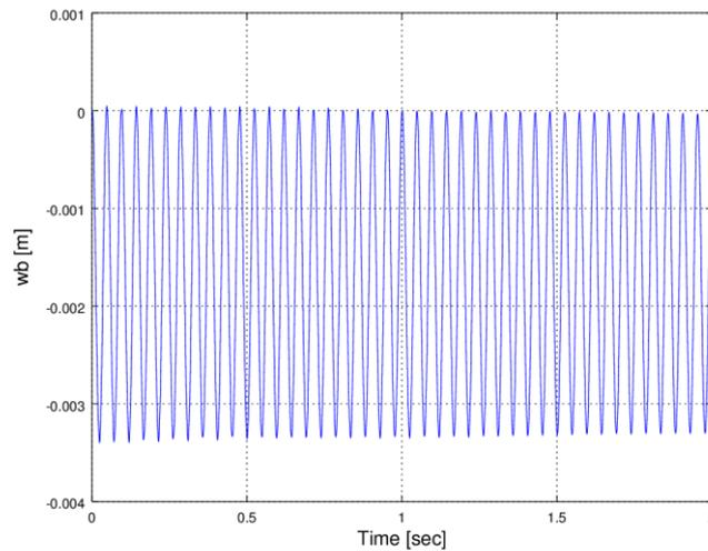
**Fig. 4 b** Dynamic mid-span  $w_b(t)$  of the numerical simply supported beam of 5 m length due to a uniform step 1 kN load, for a period of 2 seconds
