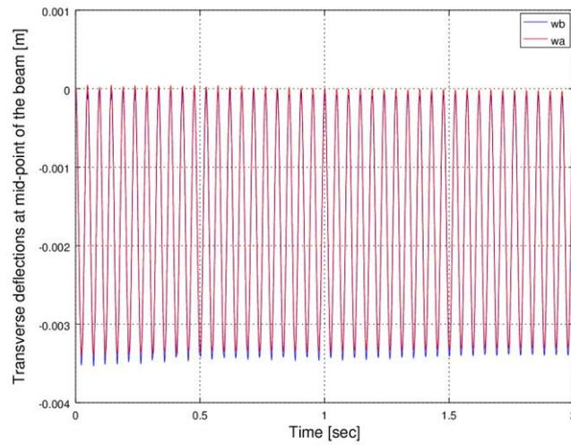
**Fig. 4 a** Dynamic mid-span transverse deflections of the numerical simply supported beam of 5 m length due to a uniform step 1 kN load, for a period of 2 seconds
