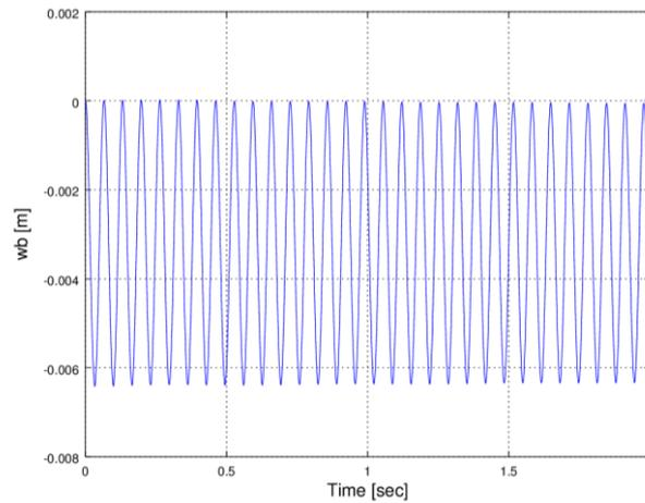
**Fig. 5 b** Dynamic mid-span  $w_b(t)$  of the numerical simply supported beam of 6 m length with  $K_n = 10^{10}$  N/m and  $K_s = 10^8$  N/m due to a uniform step 1 kN load, for a period of 2 seconds
