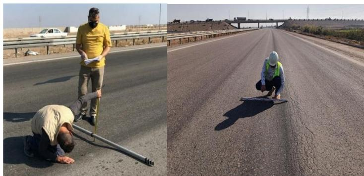
**Fig. 5 Measuring the rutted level of the three sections using Short Straight Edge Method.**
