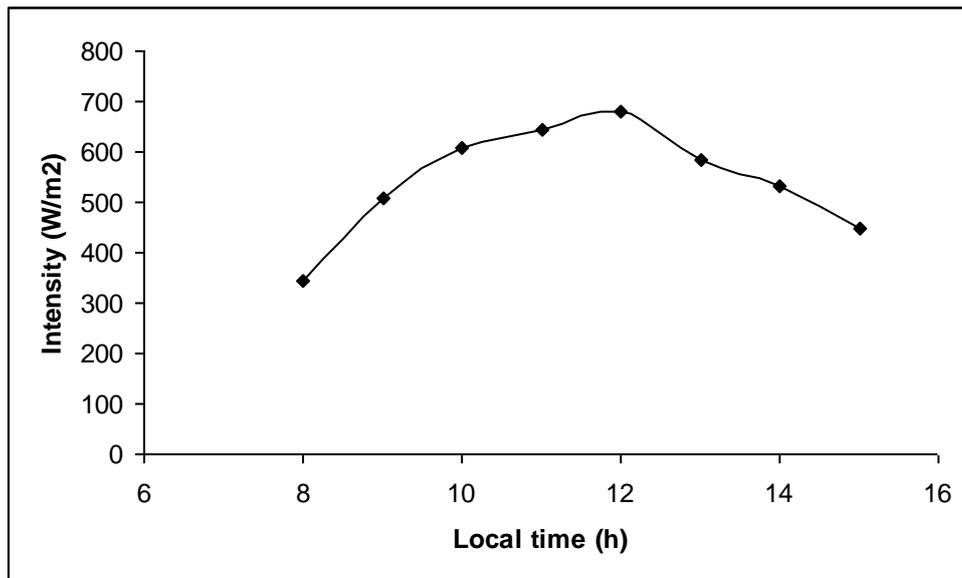
Fig.(3) : Hourly solar radiation values on tilted surface on (25<sup>th</sup> of April).
