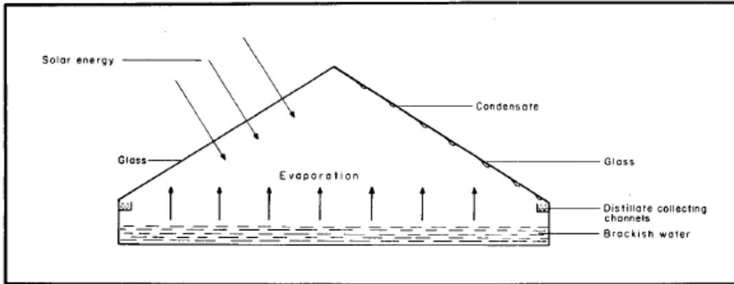
Figure (1): Schematic sketch of the solar distillation.
