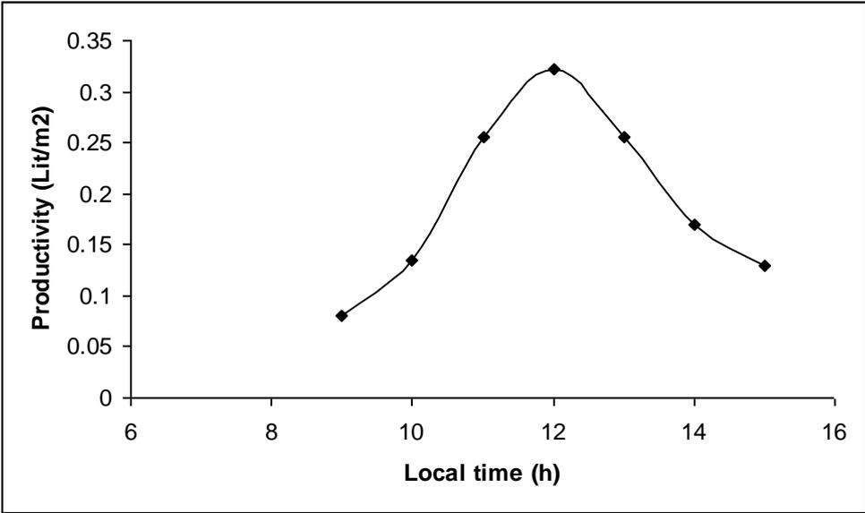
**Fig.(5): Hourly productivity of the distilled water values (25<sup>th</sup> of April).**
