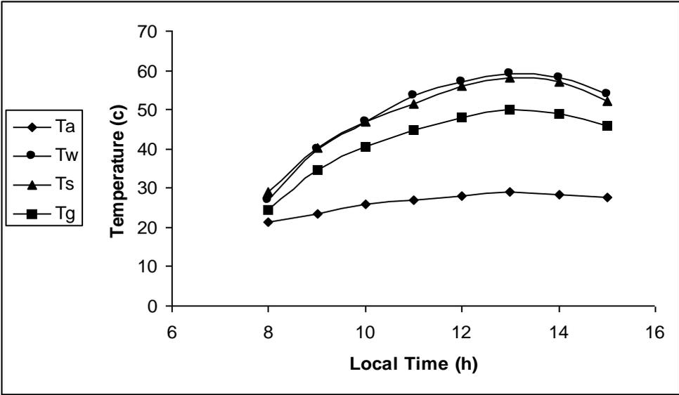
**Fig.(4): Hourly variation of temperatures values on solar still (25<sup>th</sup> of April).**
