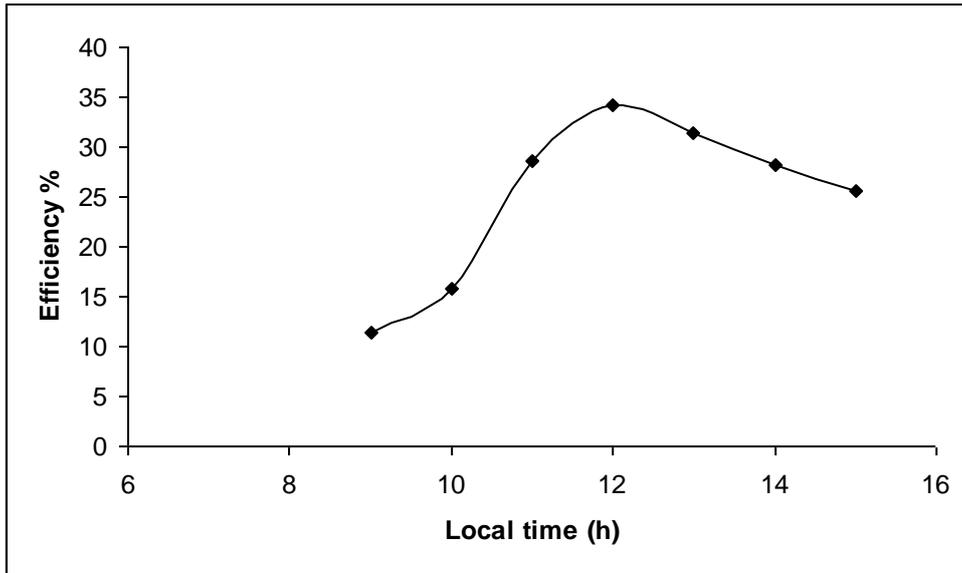
**Fig.(6): Hourly variation of the still efficiency (25<sup>th</sup> of April).**
