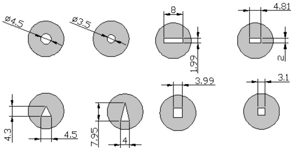
Figure (7): a schematic for the orifice plate samples
