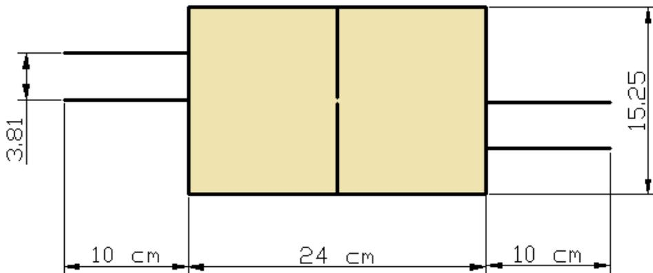
Figure (2) cross sectional area for the used silencer
