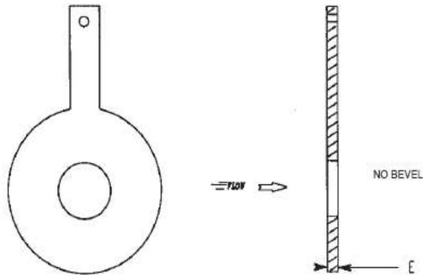
Figure (1) Restriction Orifice plate
