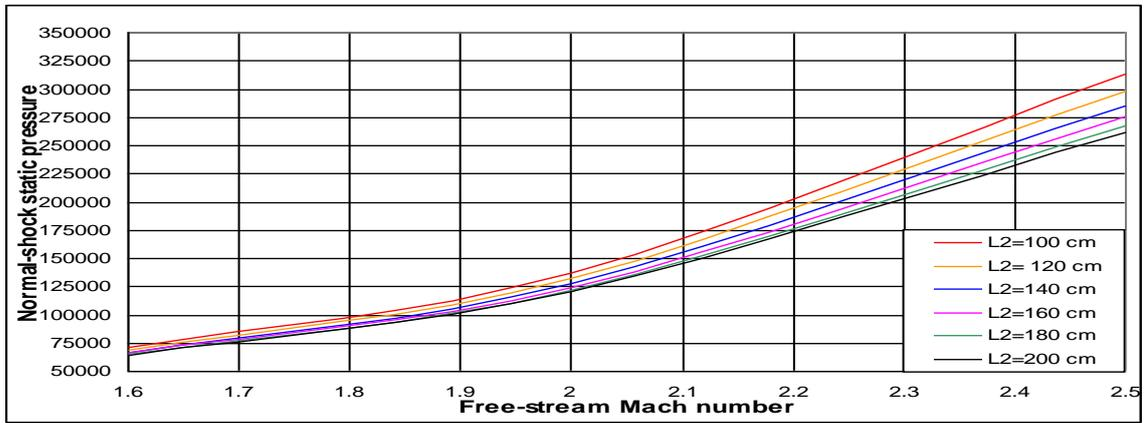
Figure (11) Static pressure downstream the normal shock versus free-stream Mach number for different nozzle divergent lengths.
