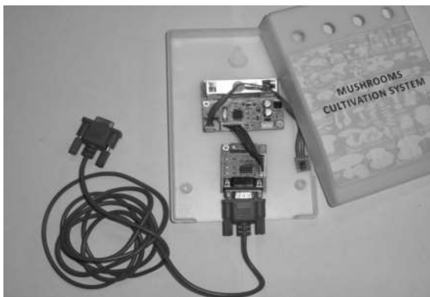
Figure (6) Sensing system and interfacing board placed in plastic cover.
