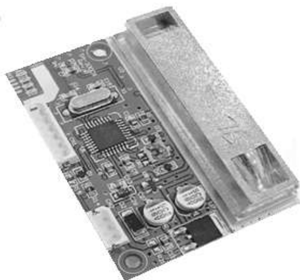
Figure (2) SH-1000-DTH NDIR dual sensor module.
