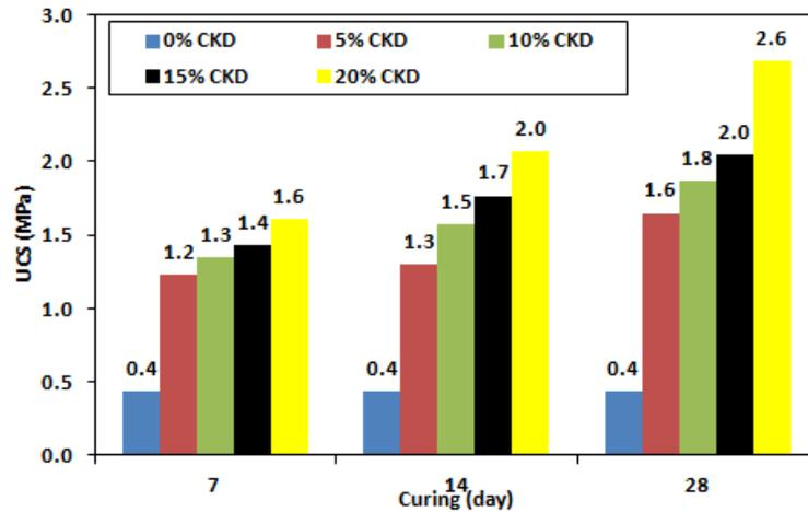
Fig. 5 UCS results for different CKD contents and cured at different periods
