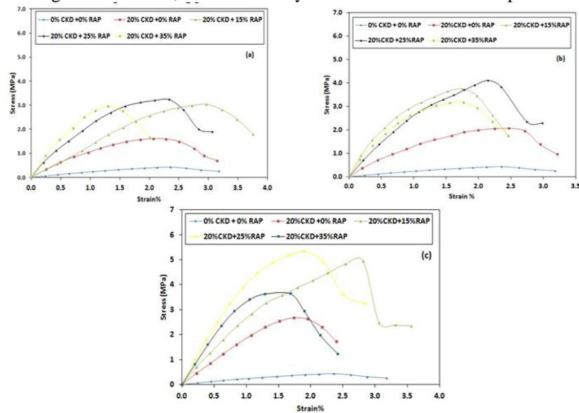
Fig. 6 Stress-strain of CKD-RAP mixture treated soil for varying curing periods: (a)7days (b)14days (c)28 days
