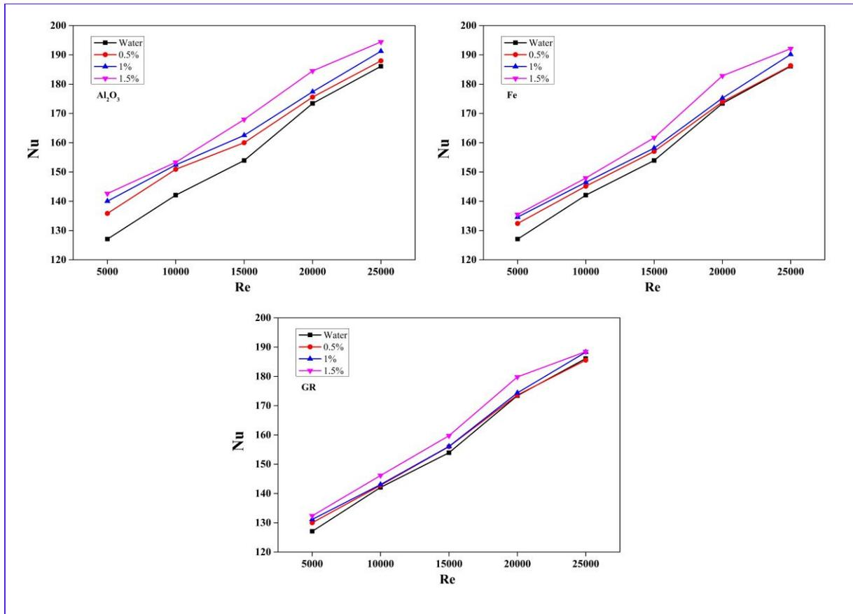
Fig. 6. Nu vs Re at all concentrations for Al<sub>2</sub>O<sub>3</sub>, Gr, and Fe-based fluids against water.
