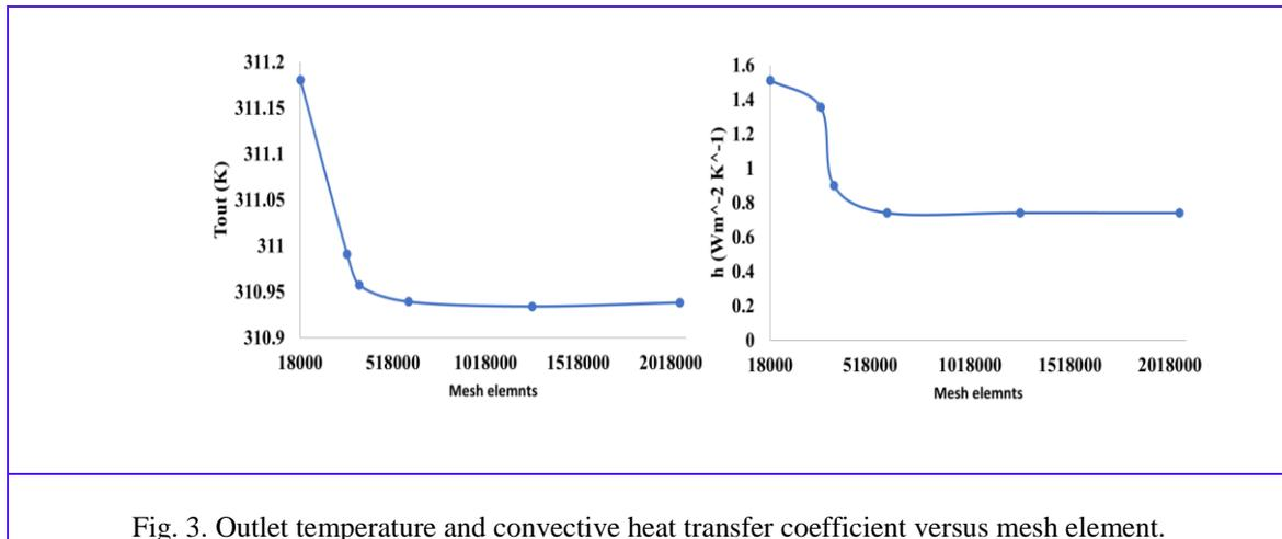
Fig. 3. Outlet temperature and convective heat transfer coefficient versus mesh element.
