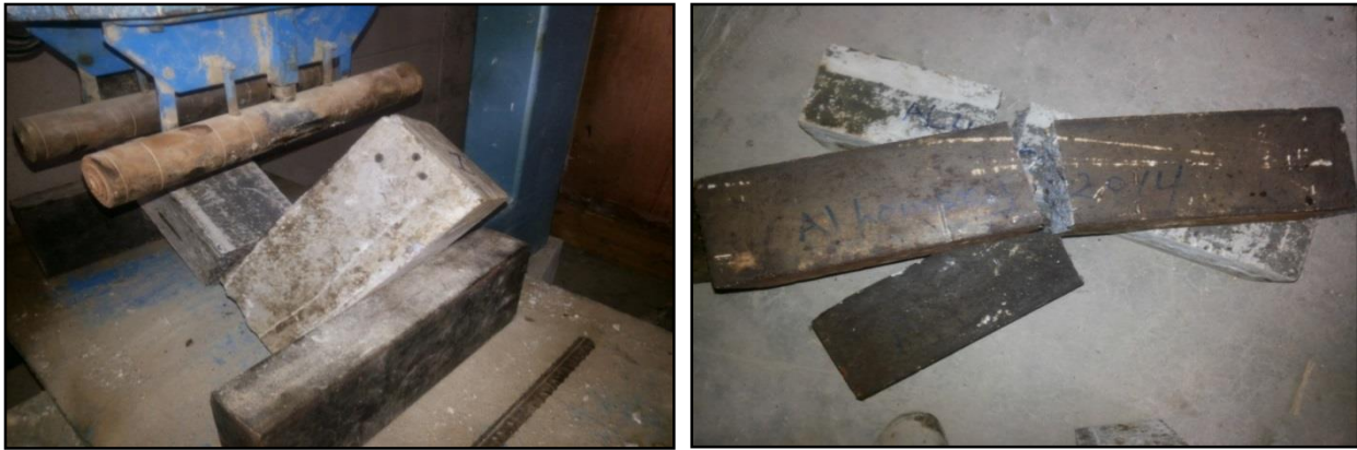
Figure 2. The modulus of rupture test
