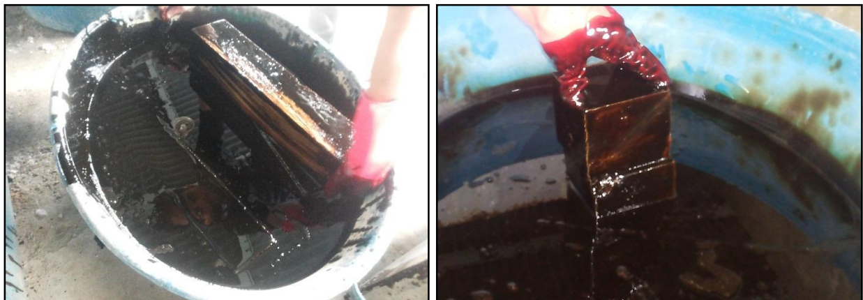
Figure 1. Specimens of concrete were subjected to a solution of concentrated crude oil.
