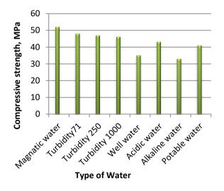
Figure 4: Varation of compressive strength with type of water at 14 days age
