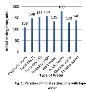
Fig. 1: Varation of initial setting time with type of
