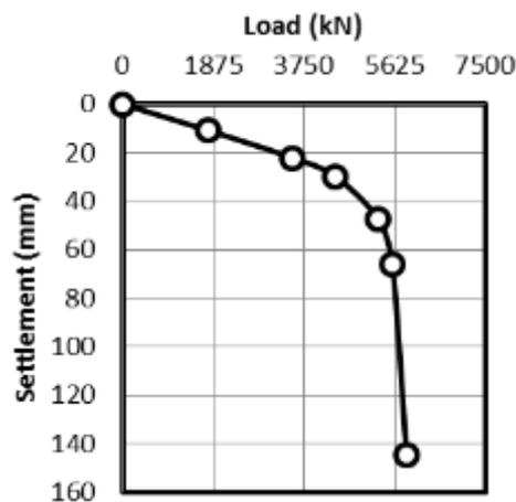
Figure (11) Load-Settlement relation of pile with D= 120 cm and L= 1800 cm.
