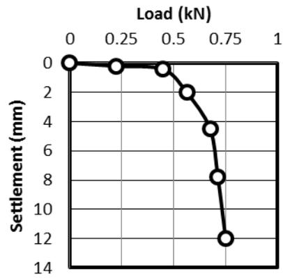
Figure (6) Load-Settlement relation of pile with  $D=4$  cm and  $L=60$  cm.
