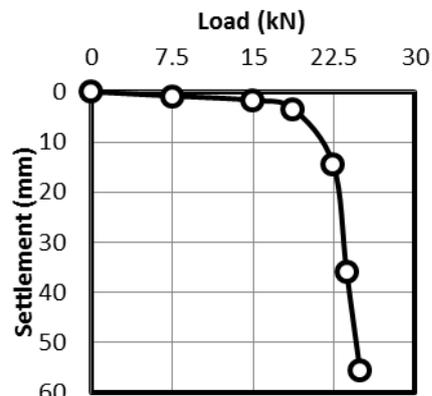
Figure (8) Load-Settlement relation of pile with D= 16 cm and L= 240 cm.
