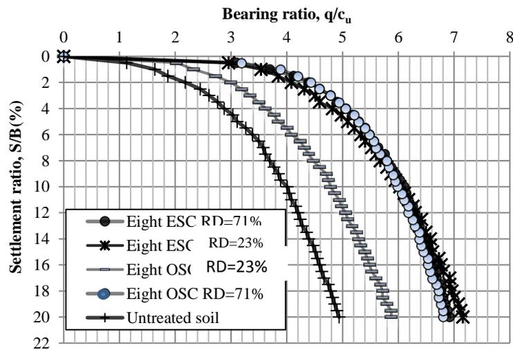
Figure (12) Bearing ratio versus settlement ratio for model test with encased stone columns.
