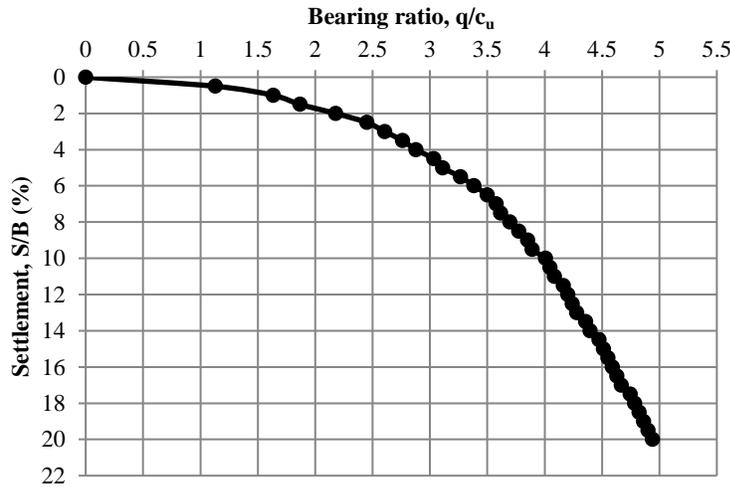
Figure (7) Bearing ratio versus settlement ratio for untreated soil.
