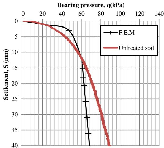
**Figure (5) Bearing pressure versus settlement for untreated soil.**
