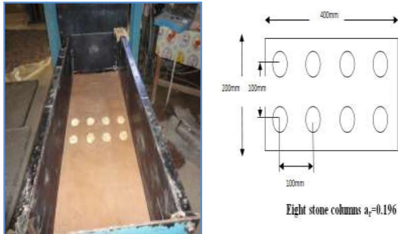
Figure (3) Stone Columns Configuration Details.
