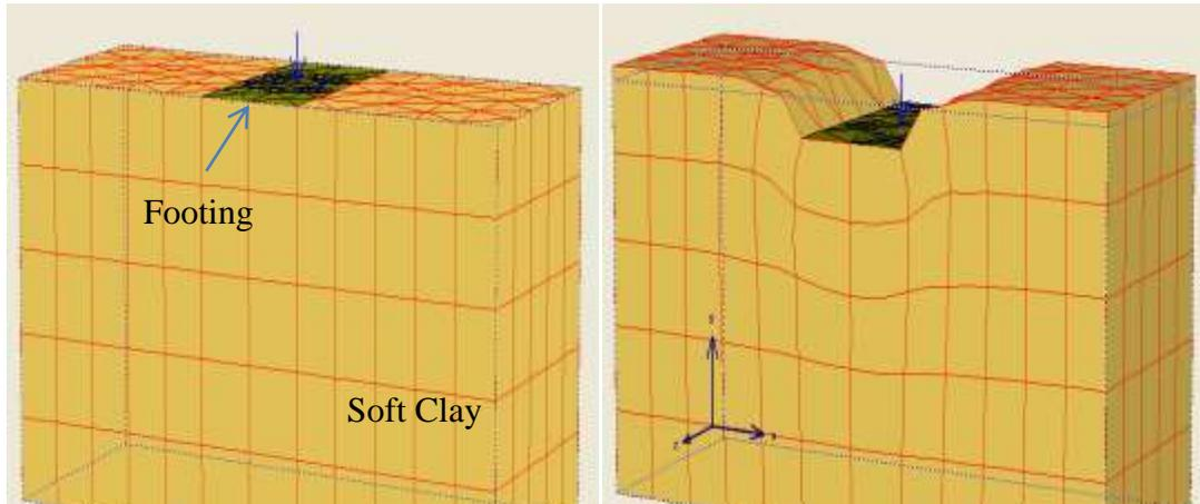
Figure (6) Finite element mesh for tested model.
