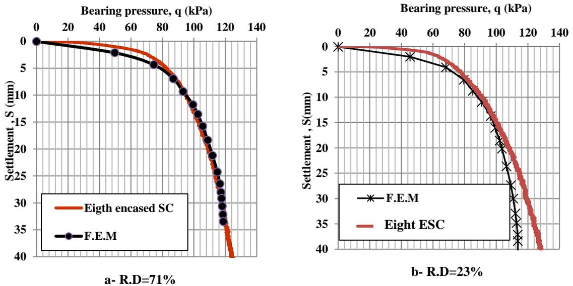
**Figure (11) Bearing capacity versus settlement for model test with encased stone columns.**
