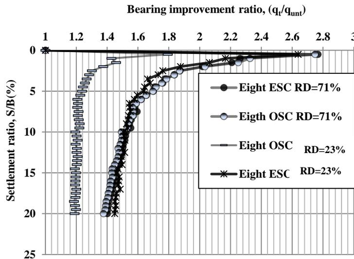
Figure (13) Bearing Improvement ratio versus settlement ratio for model test with encased.
