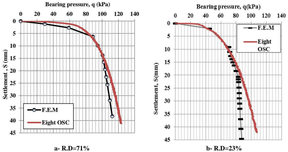
Figure (8) Bearing pressure versus settlement for model test with OSC.
