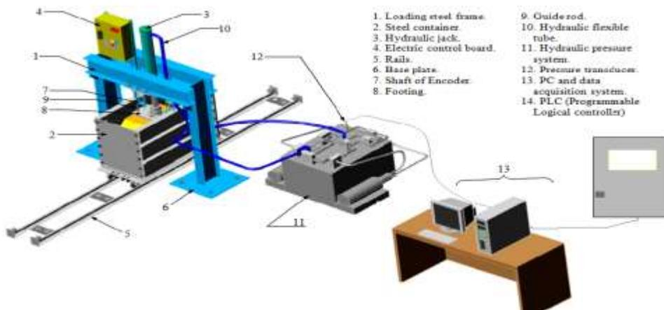
Figure (4) the general view of the apparatus.
