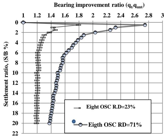
Figure (10) Bearing improvement ratio versus settlement Ratio for model tests with ordinary stone columns.
