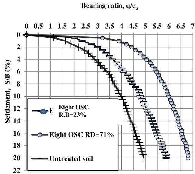
Figure (9) Bearing ratio versus settlement ratio for model tests with ordinary stone column.
