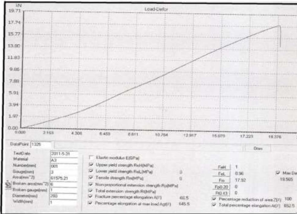
Figure (4) the values of central load ( $F$ ) vs. plate bulging ( $w_0$ ) given from testing machine for plate of thickness 3 [mm].
