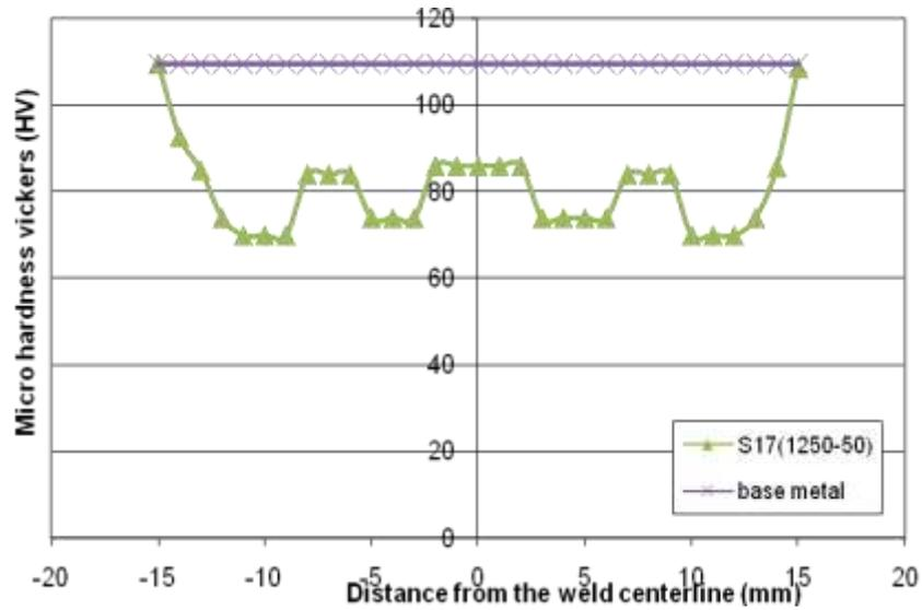
Figure (6) Microhardness profile in FSW joint welded at S17 (1250rpm-50mm/min).
