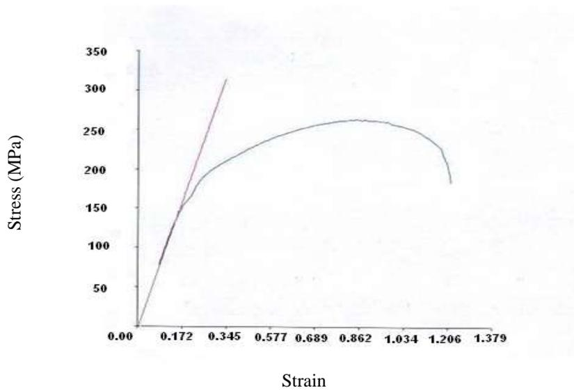
Figure (10) Stress-Strain curve for FSW joint welded at (1250 rpm/50mm/min).
