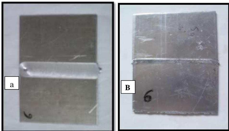
**Figure (2) Configurations FSW welded plates a- The top side of butt welded plates b- The back side of butt welded plates.**
