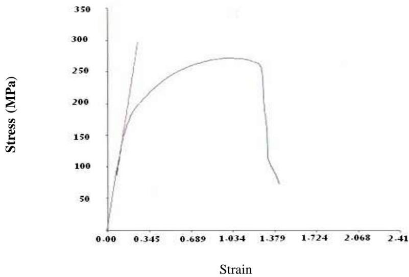
Figure (9): Stress-Strain curve for FSW joint welded at (800 rpm 125mm/min).
