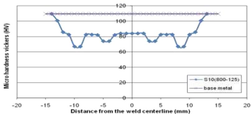
Figure (5) Microhardness profile in FSW joint welded at S10 (800 rpm-125 mm/min).
