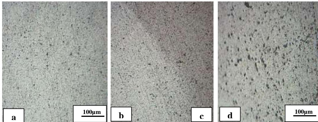
Figure (3) Microstructure of welding zones in FSW joint welded with welding parameters of (1250 rpm and 50 mm/min).
