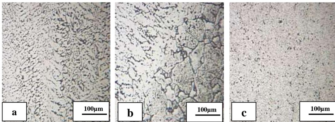
Figure (4) The microstructure of welding zones in TIG joint welded with welding current of 200 Amp, arc voltage of 12 V and welding speed of 280 mm/min: a) Weld metal b) HAZ c) base alloy.
