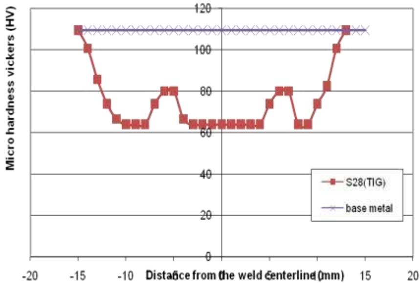
Figure (7) Microhardness profile in TIG joint (sample S28) welded at welding current (200Amp).
