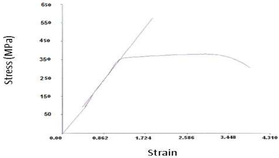
Figure (8) Stress-Strain curve for base alloy (AA 6061-T6).
