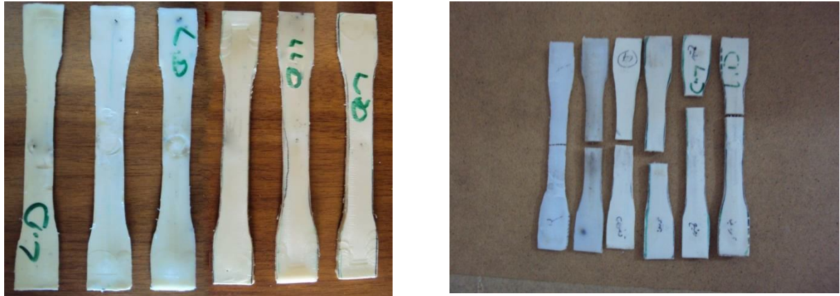
Fig.3: Samples of LDPE and LLDPE (a) before testing tensile samples, (b) after testing tensile samples
