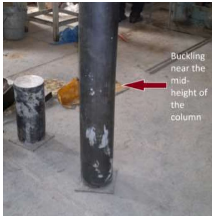
Figure. 10 Failure of the long column
