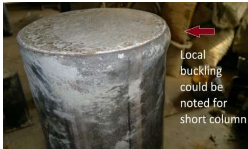
Figure. 7 Failure of the short column.
