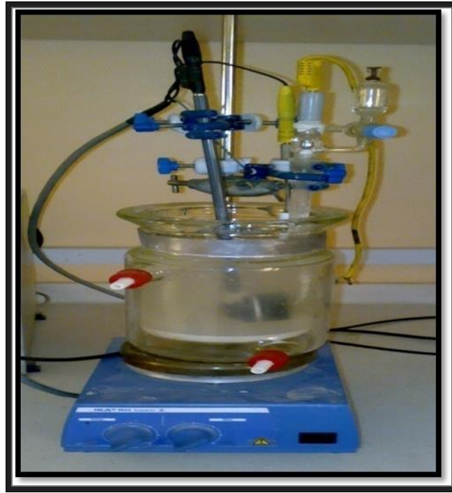
Figure 1. Photo picture shows the use of the electrochemical cell in drawing polarization curves.
