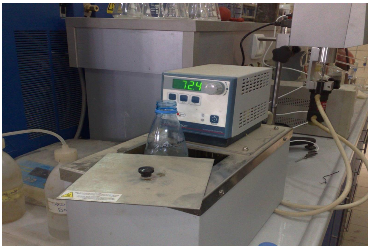
Figure (2) DV-II+Pro viscometer with temperature bath
