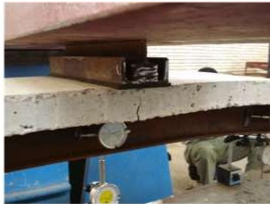
(b) Tension cracks at region of max. +ve moment, front view.
