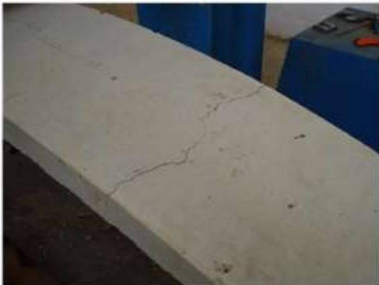
(c) Transverse crack at max. -ve moment & longitudinal cracks at right side.
