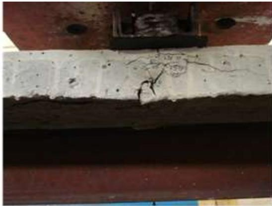
(a) Tension cracks & concrete crushing at region of max. +ve moment, rear
