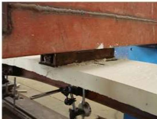
(c) Concrete crushing at region of max. +ve moment, top surface.
