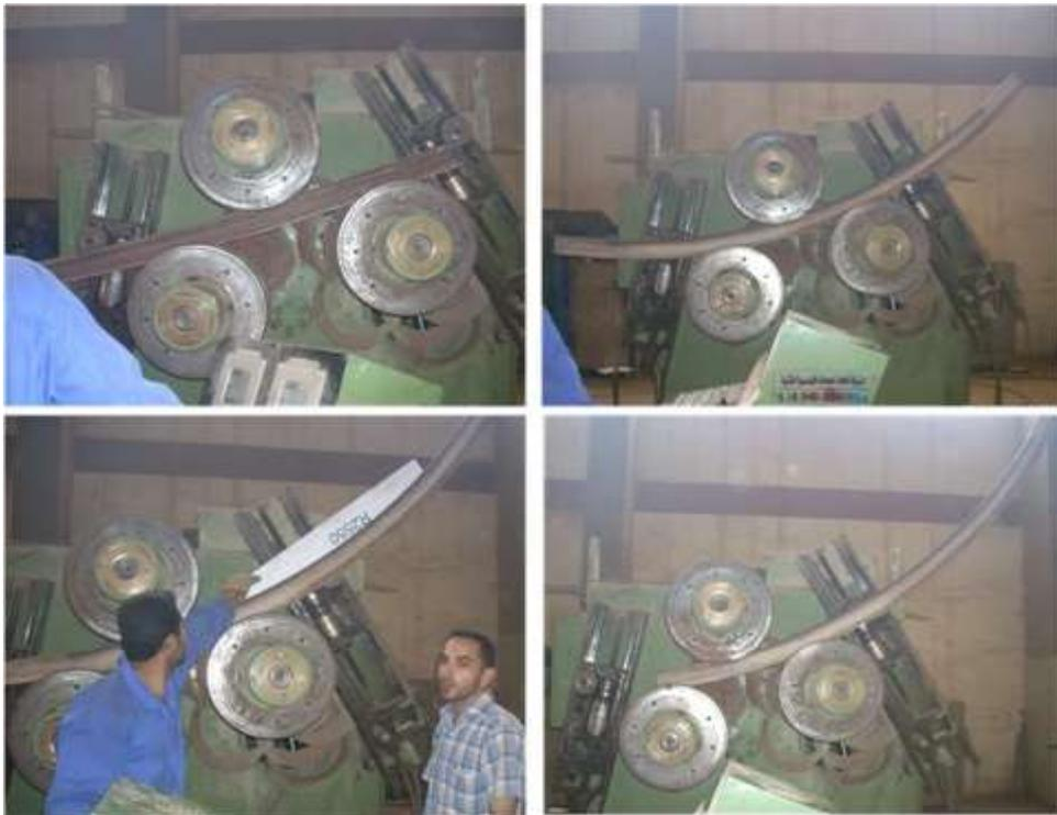
Figure (6) Photos of curving (bending) process.
