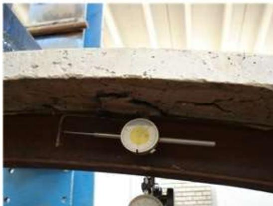
(f) Longitudinal cracks at left side, bottom surface.
