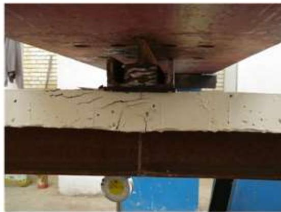
(b) Tension cracks at region of max. +ve moment, rear view.
