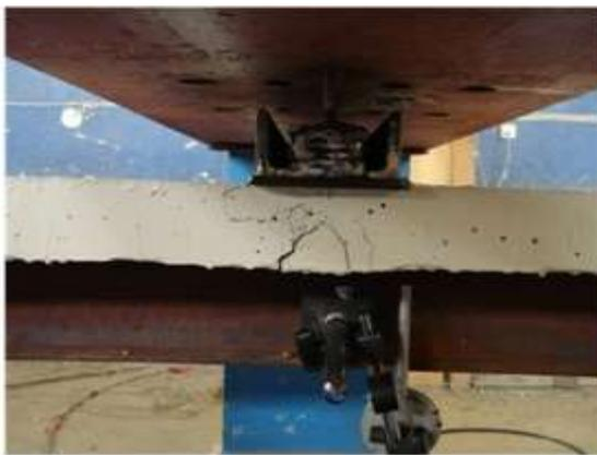
(a) Tension cracks & concrete crushing at region of max. +ve moment, front
