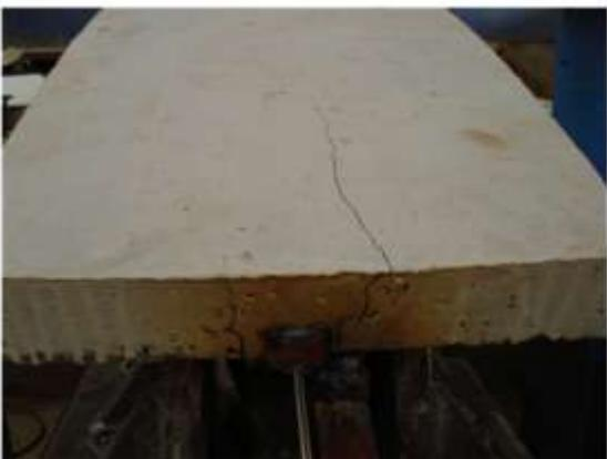
(e) Longitudinal cracks at left end.
