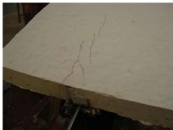
(f) Longitudinal cracks at right end.
