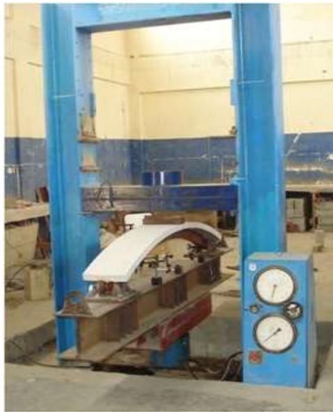
Figure (8) Photo of universal testing machine.
