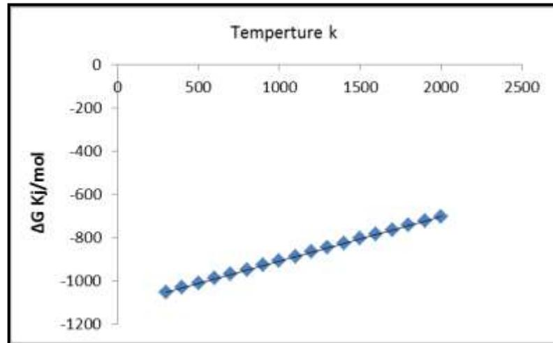
**Figure (4) Relationship between Gibbs free energy and reaction temperature [10].**
