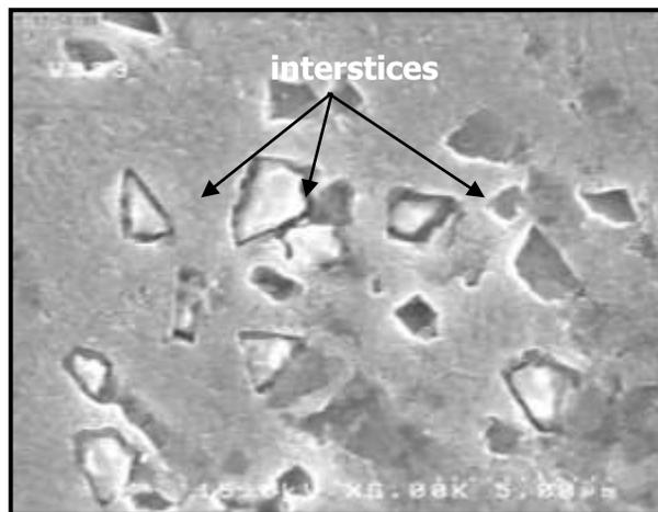
Figure (9) SEM image illustrated interstices around alumina particles.
