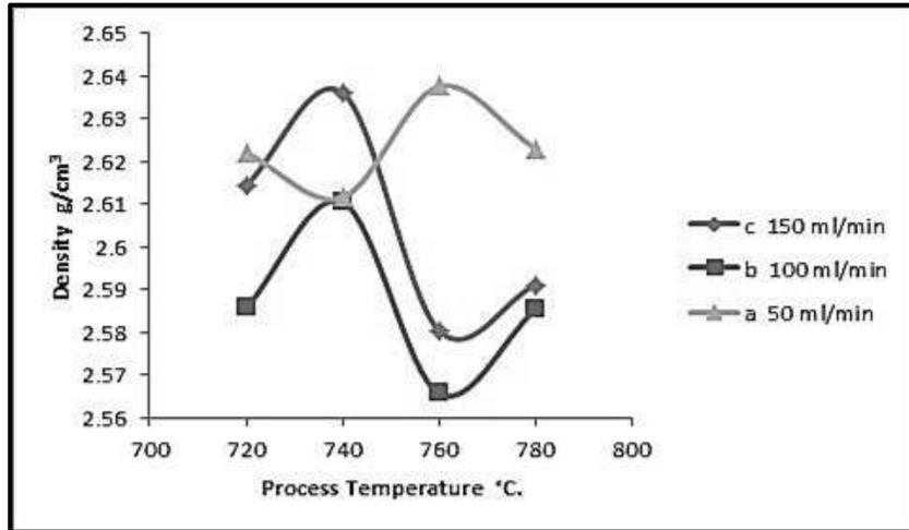
Figure (8) Relationship between density and reaction temperature °C.
