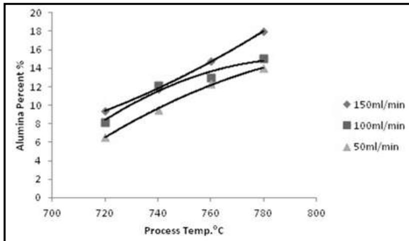
Figure (7) The relationship between alumina percent and reaction temperature °C.
