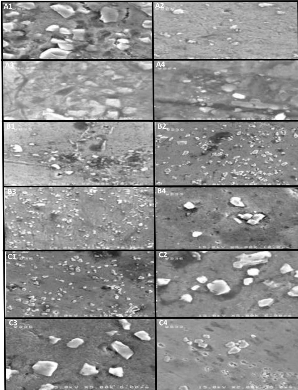
Figure (5) SEM images for samples A, B, C at oxygen gas flow rate 50, 100, 150 ml/min respectively and 1, 2, 3 and 4 at reaction temperatures 780,760,740,720<sup>o</sup>C respectively.
