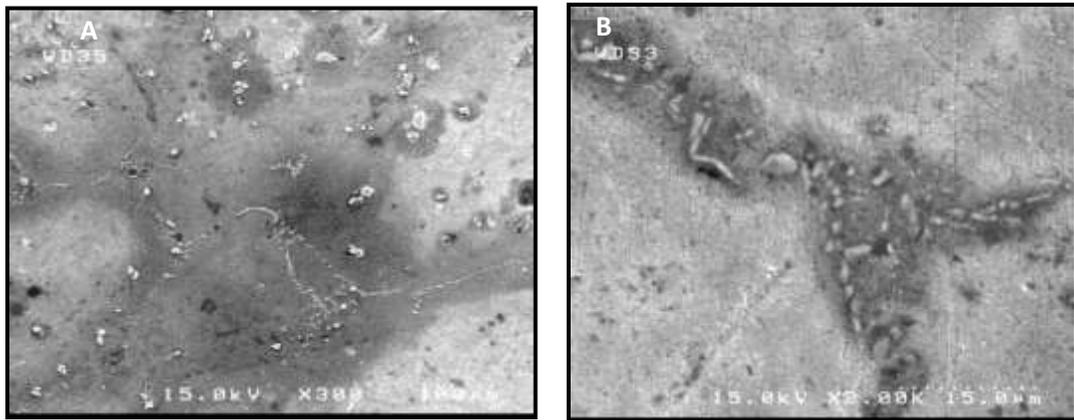
Figure (11) SEM images illustrated alumina particles (A) segregation and (B) agglomeration at grain boundaries.
