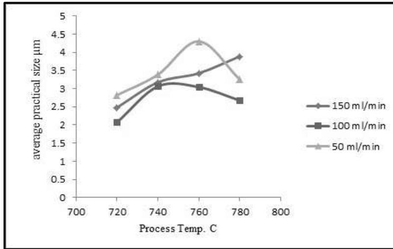
Figure(6) Relationship between alumina average practical size (µm) and reaction temperature (°C).
