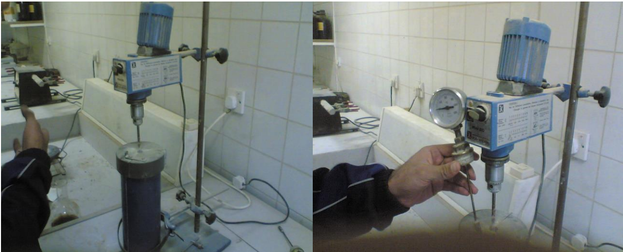
Fig. 1: Measuring the temperature of reaction of lime and aluminum.
