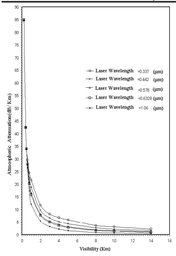
Figure (1) Atmospheric attenuation as a function of the visibility for different laser wavelength.
