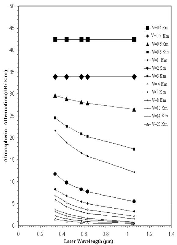
Figure (2) Atmospheric attenuation as a function of laser wavelength for different visibility (V) in kilometer unit (Km).
