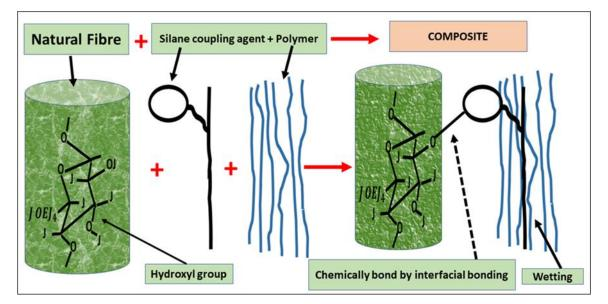
Figure 2: Schematic representation of silane treatment.
