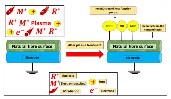
Figure 3: Schematic representation of the plasma surface treatment.
