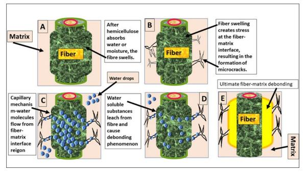
Figure 1: Schematic Representation of Effect of Water on Fiber-Matrix Interface.
