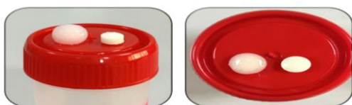
Figure 4. Swelling of tablets after 4 hrs of disintegration test
