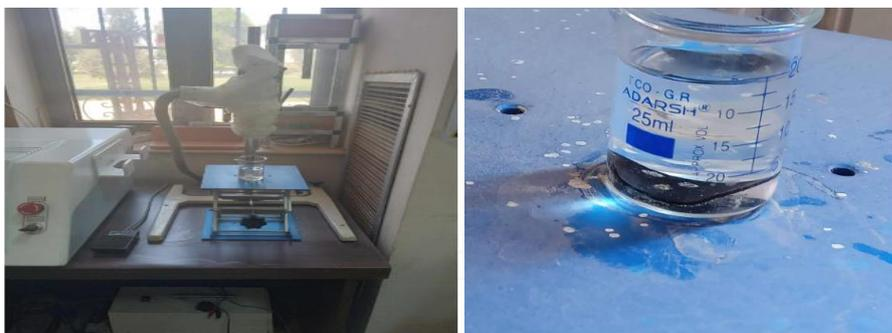
Figure 2: Creation of graphene oxide (GO) via laser ablation from graphite
