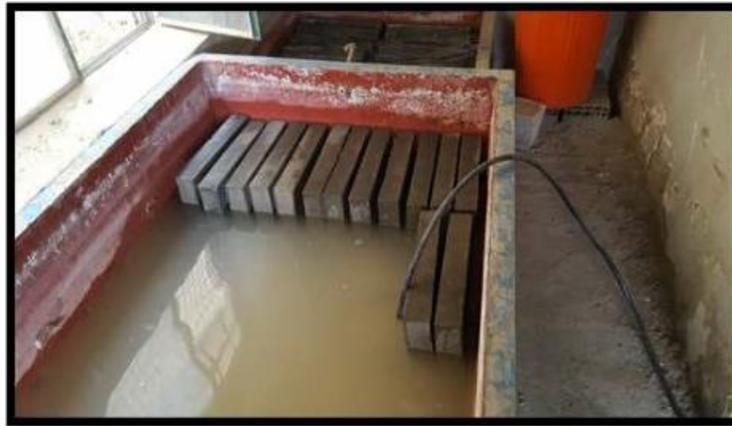
Figure 6. Slabs during curing.
