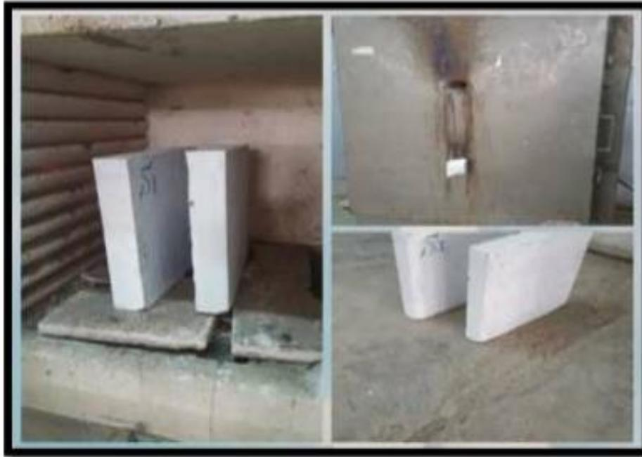
Figure 9. Slab specimens within the electric furnace
