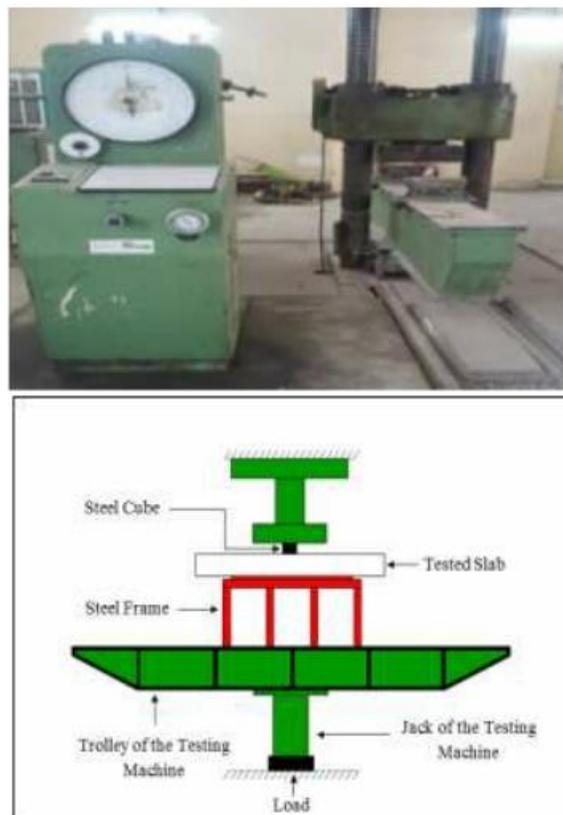
Figure 7. The universal testing machine with hydraulic motion.
