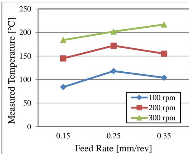
**Figure 7** The variation of temperature with respect to feed rate at tool of 110° point angle.
