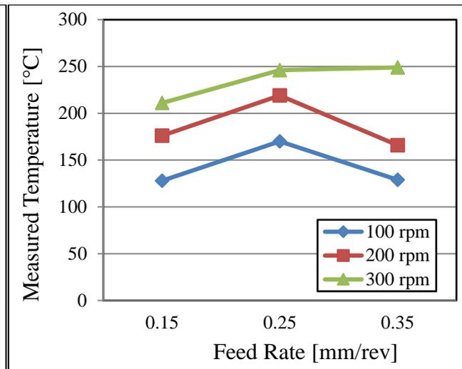
**Figure 8** The variation of temperature with respect to feed rate at tool of 118° point angle.
