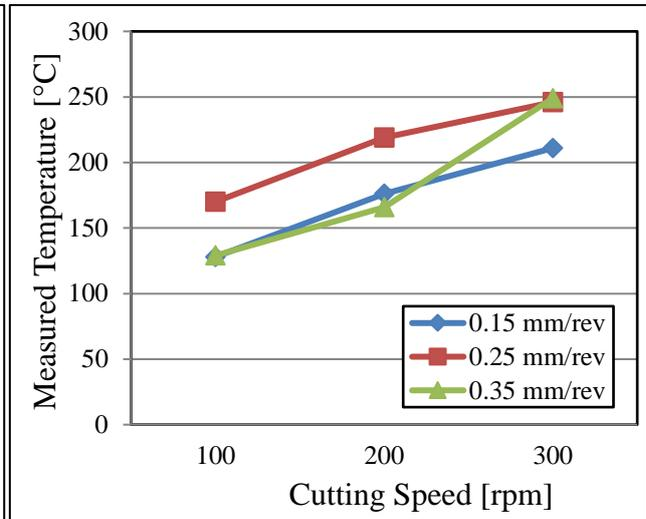
**Figure 6 The variation of temperature with respect to cutting speed at tool of 118° point angle.**
