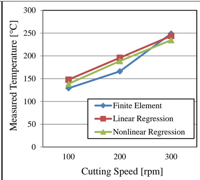
**Figure 16** The variation of temperature vs. cutting speed for a feed of 0.35 mm/rev, tool 118°.
