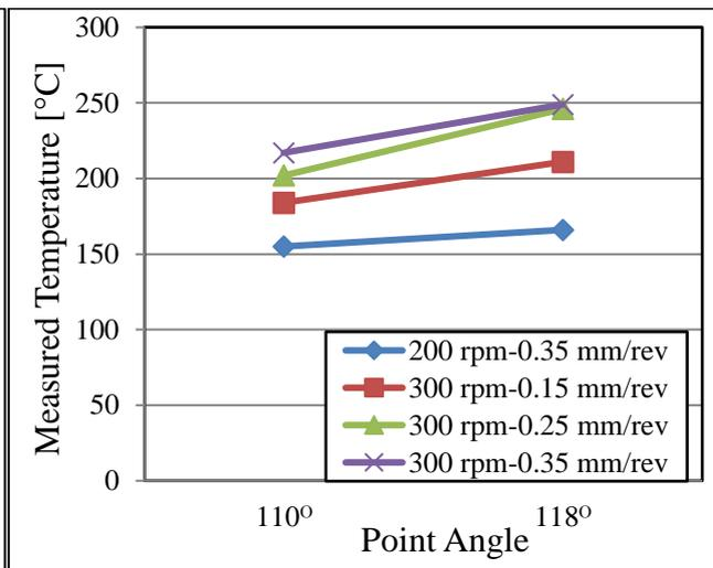
**Figure 10 The variation of temperature with respect to point angle for four FE operations.**
