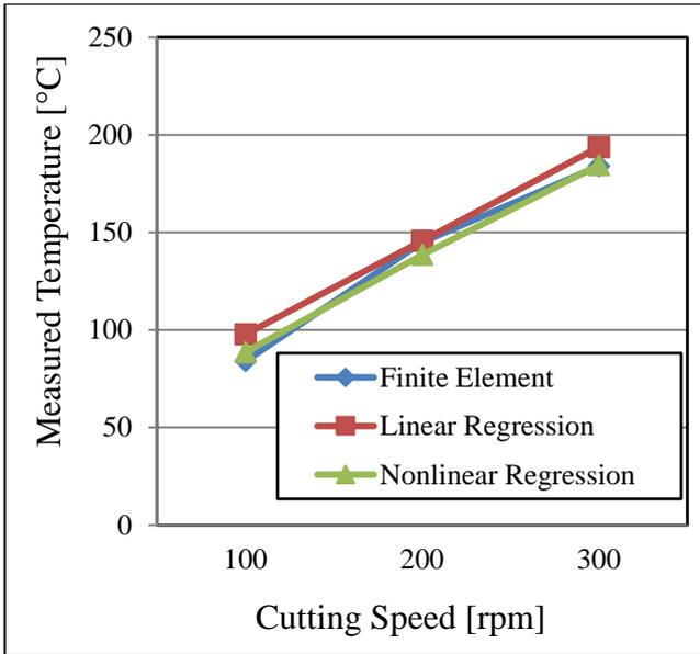
**Figure 11** The variation of temperature vs. cutting speed for feed of 0.15 mm/rev, tool 110°.
